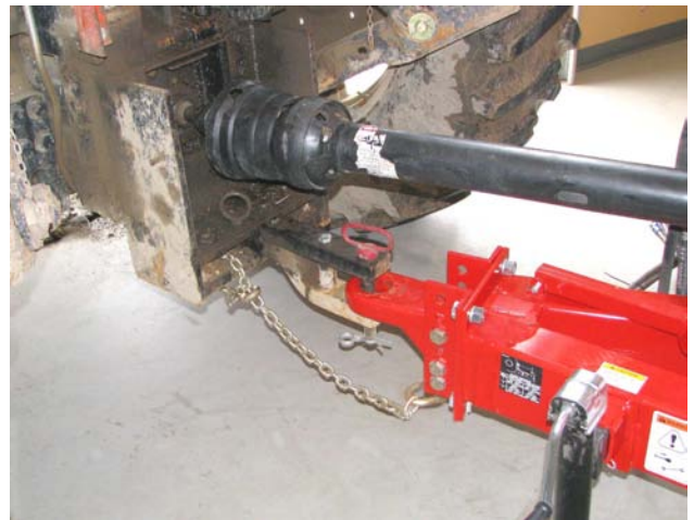
Remove Driveline and Safety Chain
