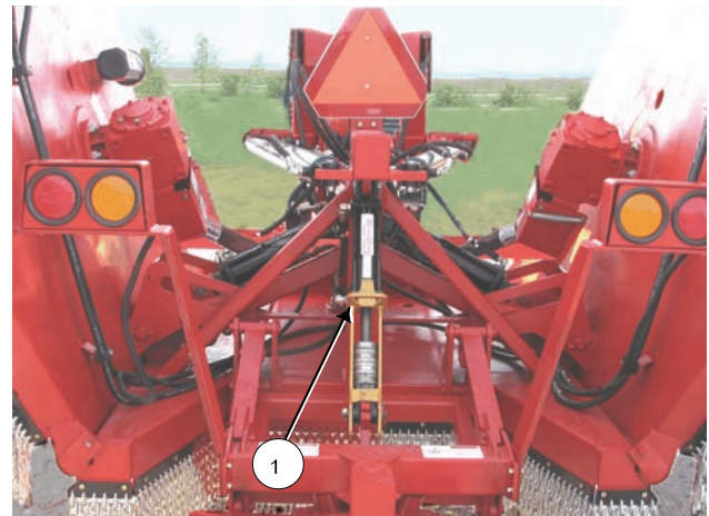
Height Cylinder Resting on Lock
