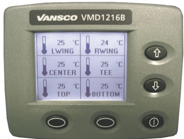
Monitor Gearbox Temperatures
