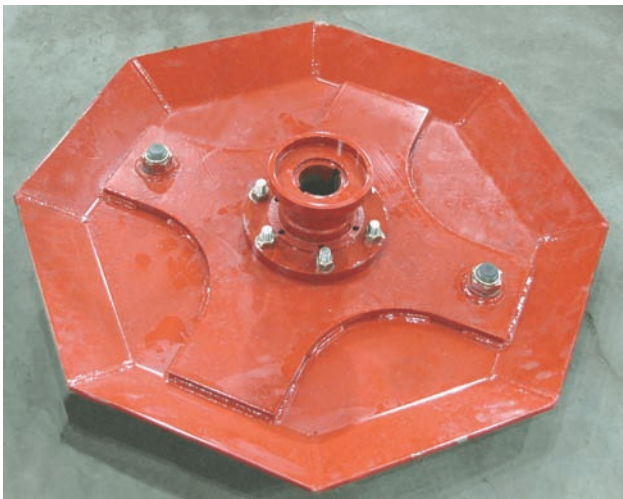
Blade Pan Removed
