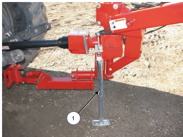
Single Point Hitch on Jack
