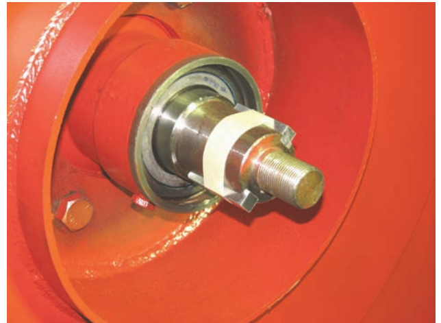
Keys Taped Onto Driveshaft
