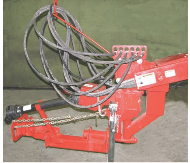
Hydraulic Hoses, PTO and Connector
