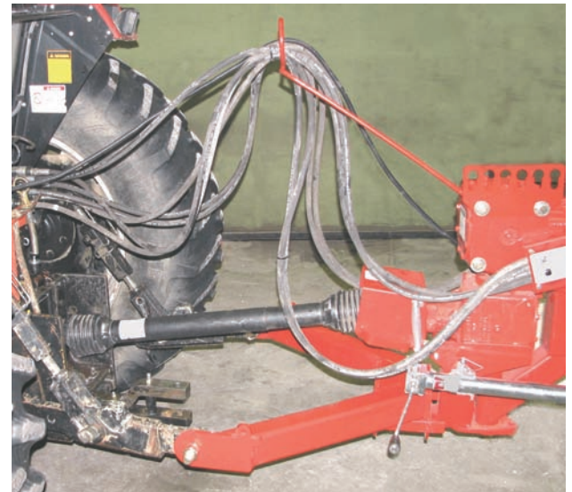
2 Point Hitch Connection
