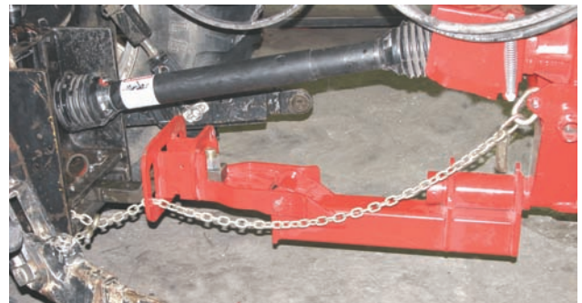
Remove Driveline and Safety Chain
