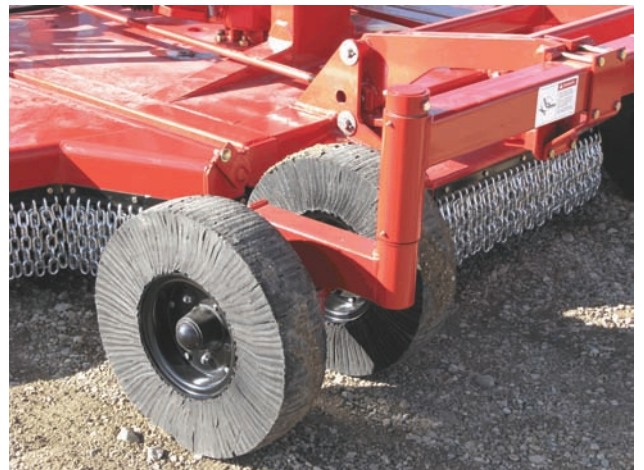
Check Condition of the Chain Guards
