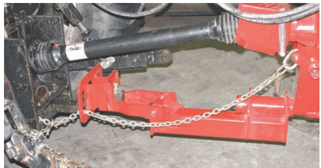
Attach Driveline to PTO
