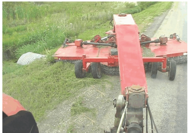
Rotate Mower Away from Obstructions
