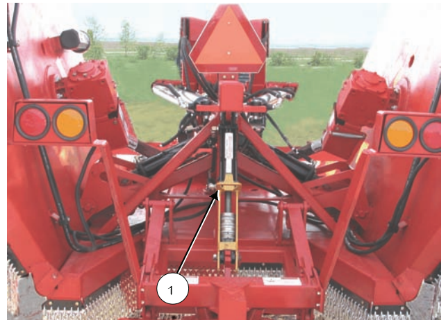
Height Cylinder Resting on Lock
