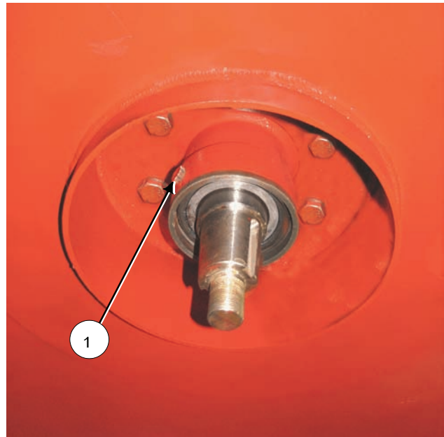
Splitter Box Oil Drain Plug
