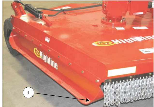
Inspect Skid Shoe
