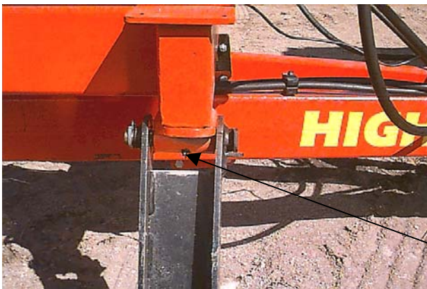
Figure 3 - Pivot Arm Grease Location
