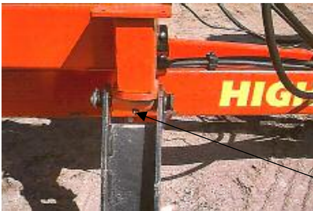
Figure 3 - Pivot Arm Grease Location
