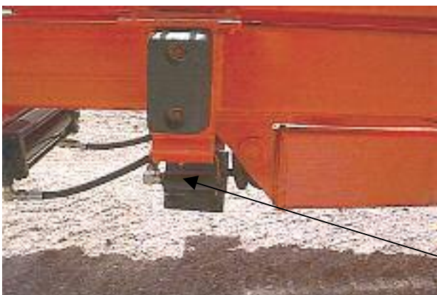
Figure 4 - Pivot Slide Arm Grease Location
