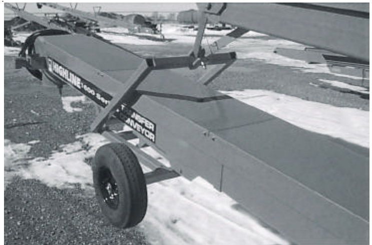
Figure 21 Raise undercarriage to tighten carrier linkage
