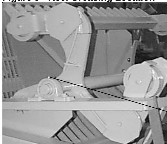
Figure 5 - Reel Greasing Location
