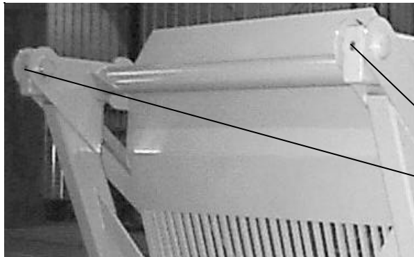
Figure 7 - Dump Mechanism Grease Locations
