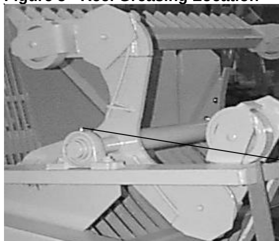
Figure 5 - Reel Greasing Location
