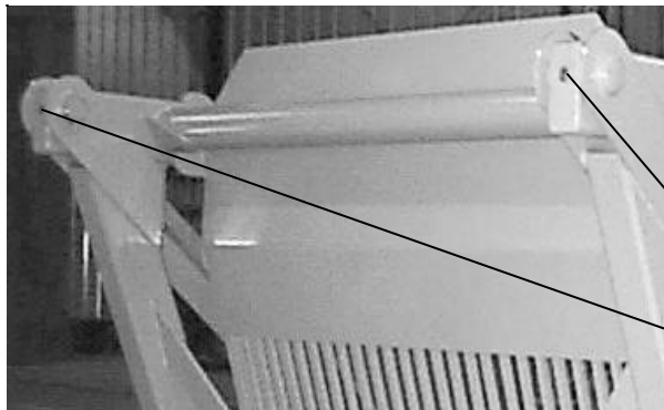
Figure 7 - Dump Mechanism Grease Locations
