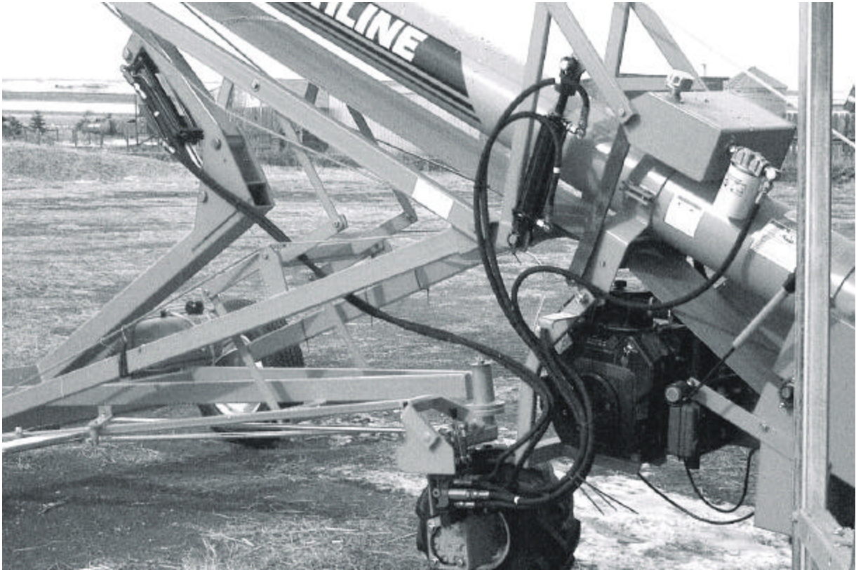
Hydraulic Hose Routing
