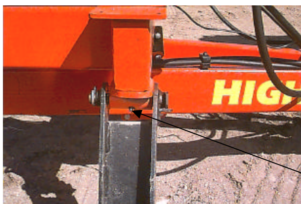
Figure 3 - Pivot Arm Grease Location
