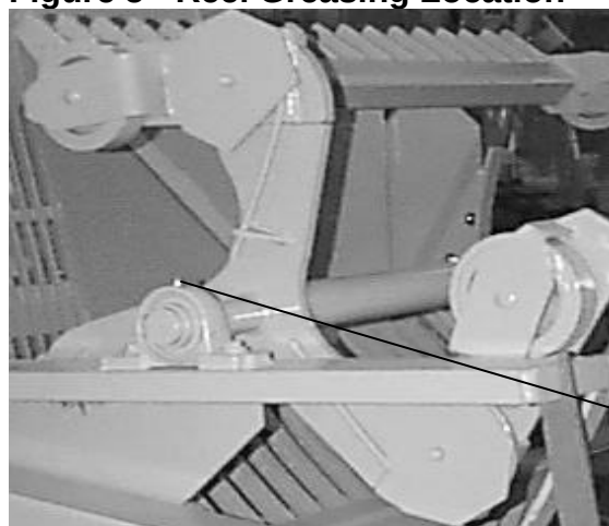
Figure 5 - Reel Greasing Location
