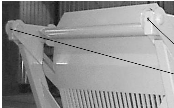
Figure 7 - Dump Mechanism Grease Locations
