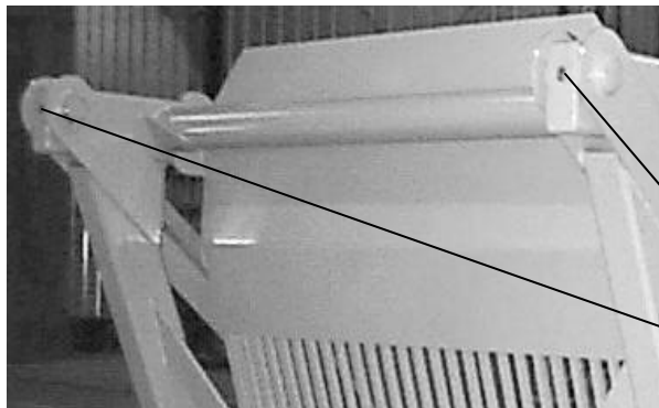
Figure 7 - Dump Mechanism Grease Locations
