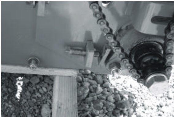
Figure 1.2(a) Belt Tracking Adjustment - Intake
