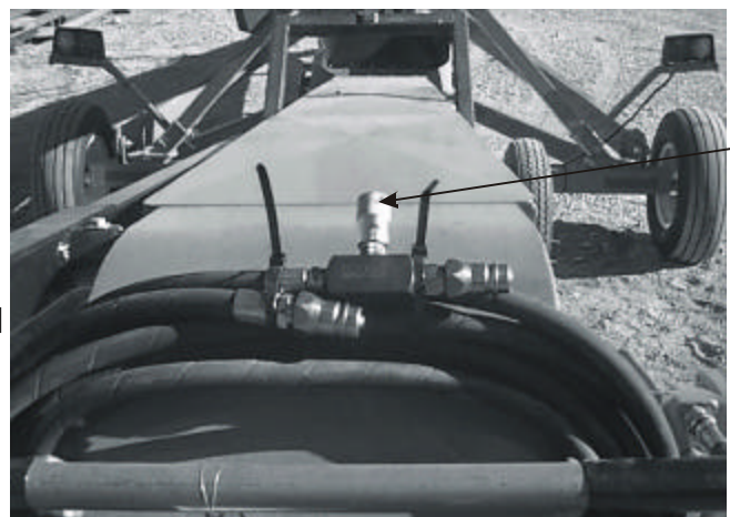
Figure 7 Flow control - turn out for maximum belt speed
