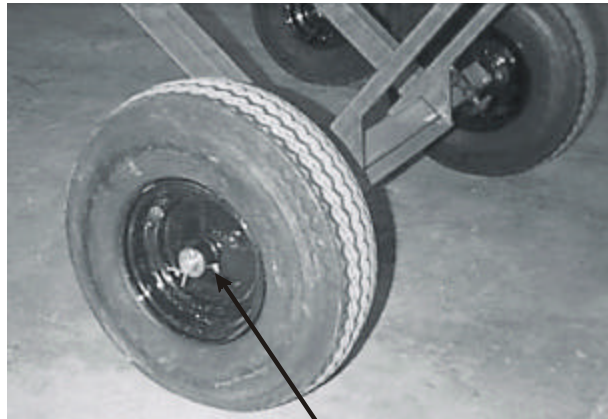
Figure 3 Main wheel grease location - 200 hours
