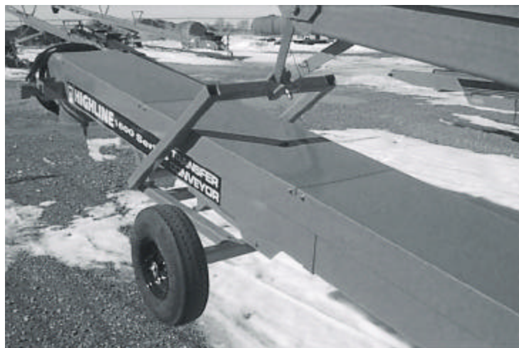
Figure 21 Raise undercarriage to tighten carrier linkage
