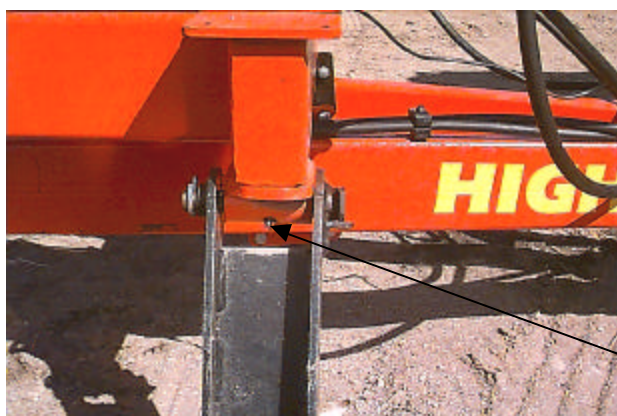
Figure 3 - Pivot Arm Grease Location
