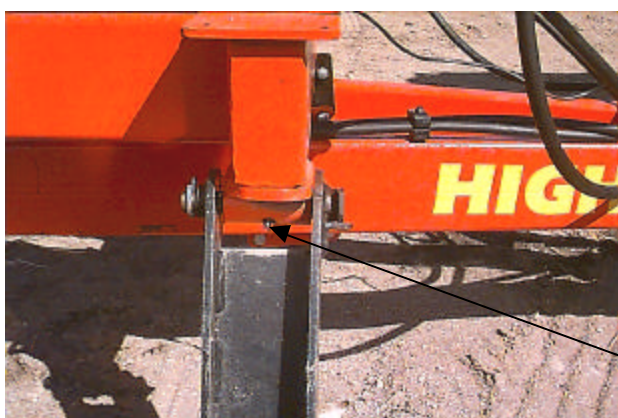
Figure 3 - Pivot Arm Grease Location
