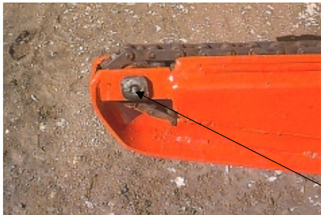
Figure 6 - Rear Sprocket Pin
