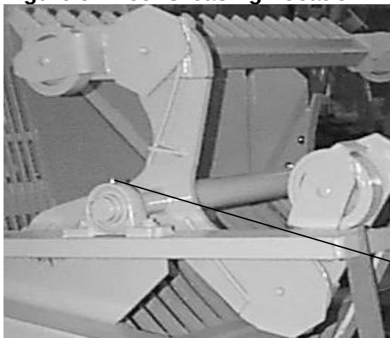
Figure 5 - Reel Greasing Location
