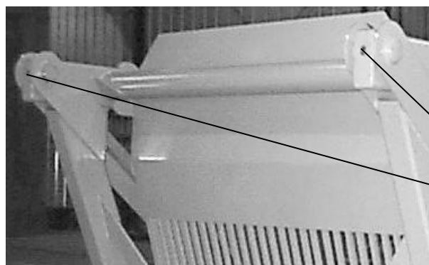
Figure 7 - Dump Mechanism Grease Locations
