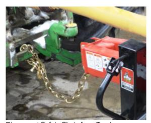
Disconnect Safety Chain from Tractor 224203 Remove the Hitch Pin
