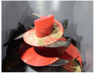
Check for Build Up in the Tub and the Condition of the Screw 224178
