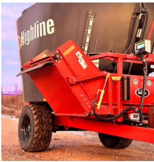
Raise the Hydraulic Folding Conveyor <sup>224181</sup> (RH Hydraulic Folding Conveyor Shown)
