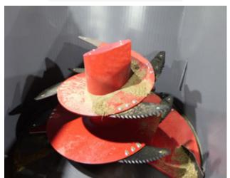
Check that the Mixing Screw Turns
