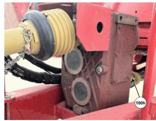
Grease Driveline Going Out of the Optional Manual Shift 2-Speed Gearbox
