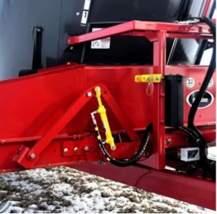
Check All Hydraulics (RH Hydraulic Folding Conveyor Shown)
