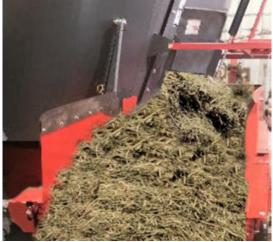
Open the Tub Door to Control Flow of Mixed Material
