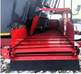
Start the Unload Conveyor (RH Hydraulic Folding Conveyor Shown)
