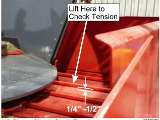
Lift Slat to Check Chain Tension
