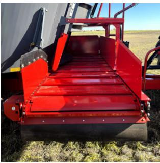
Check that the Unload Conveyor Works (RH Hydraulic Folding Conveyor Shown)
