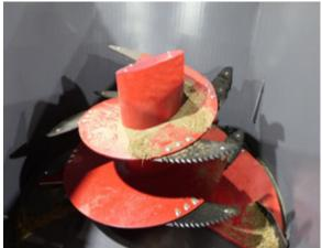
Turn Off Screws When Tub Is Empty
