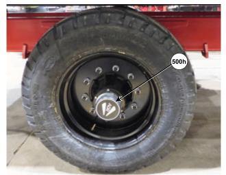
Grease the Single Axle Hubs
