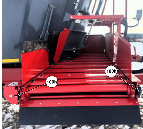
Grease Conveyor Front Bearings (RH Hydraulic Folding Conveyor Shown)
