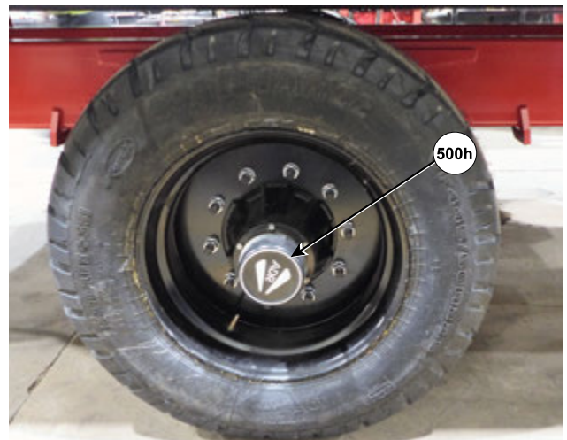
Grease the Single Axle Hubs
