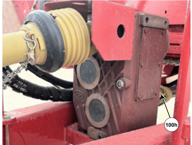
Grease Driveline Going Out of the Optional Manual Shift 2-Speed Gearbox 224147C2
