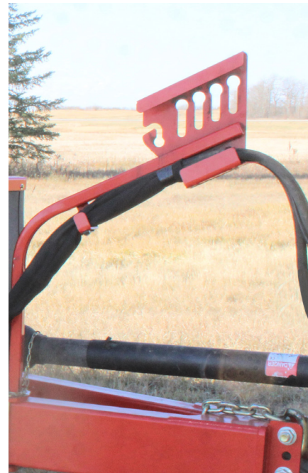
Figure 18: Route the hoses through the abrasion sleeve and into the hose holder
