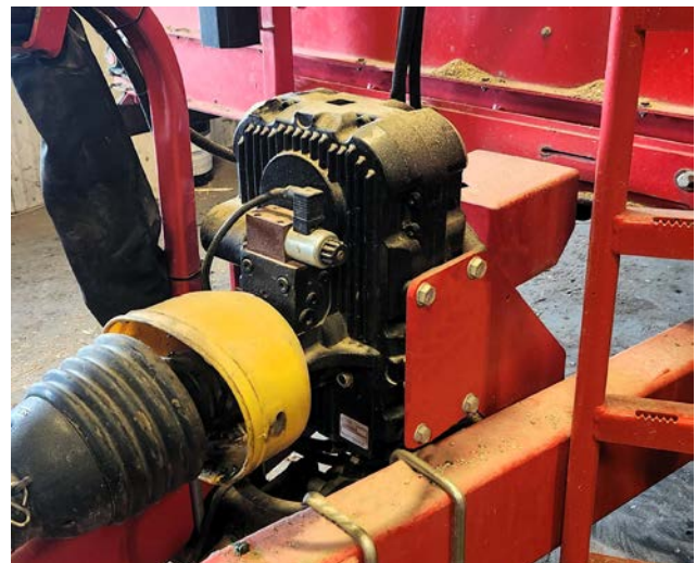
Figure 10: Connect the PTO to the gearbox 225044
