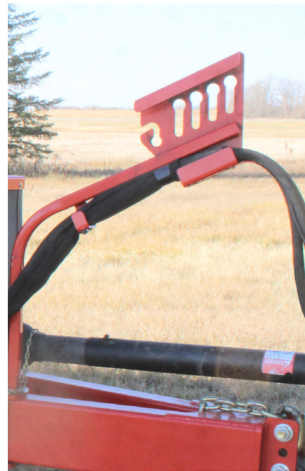
Figure 23: Route the hoses through the abrasion sleeve and into the hose holder
