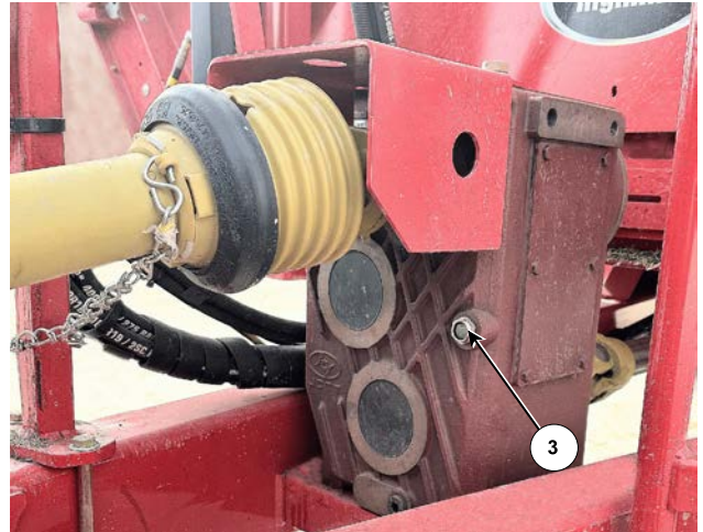
Figure 9: Check the Oil Level in the Gearbox 224173C4
