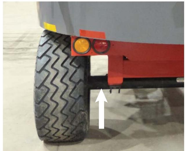
Place Jack Under the Spindle Tube of Tire to be Changed
