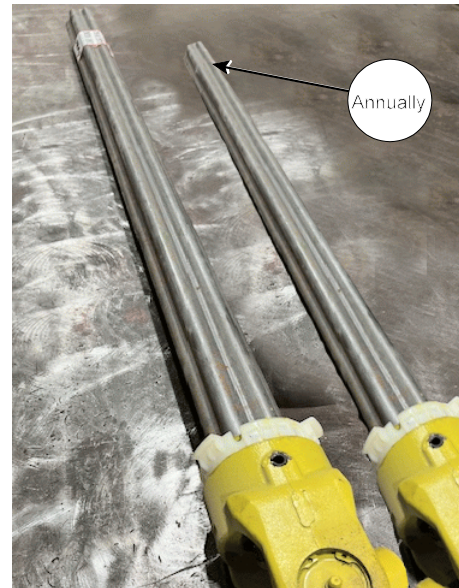
Grease the Sliding Portion of the Driveline to the Screw Drivebox 224131C
