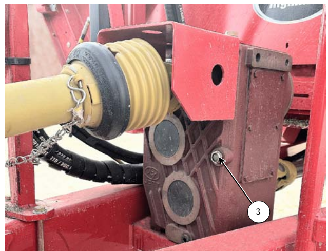
Check the Oil Level in the Optional 2 Speed Gearbox
