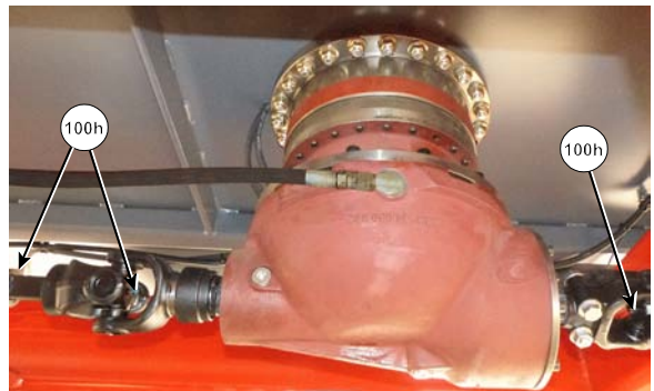
Front Screw Driveline (Corner Drivebox Shown)
