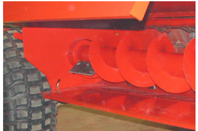
Remove Twine From Auger
