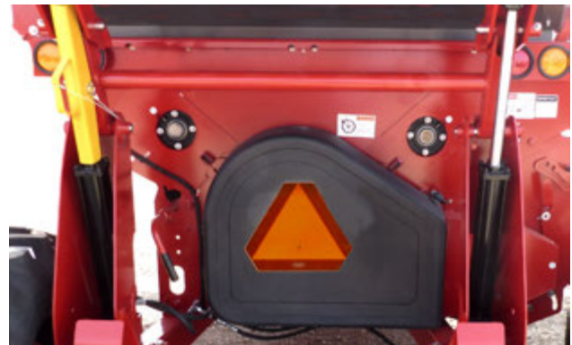
Close the Rear Drive Shield
