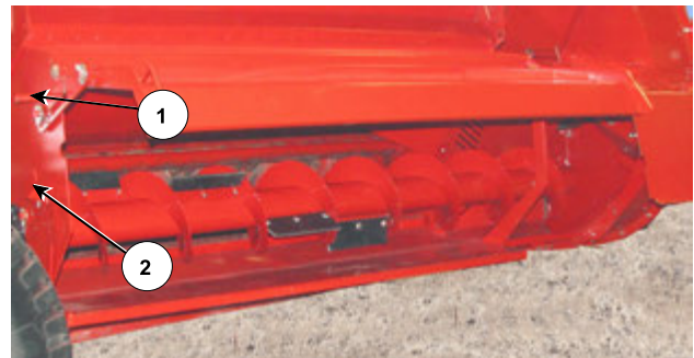
Open the Auger Housing Doors
