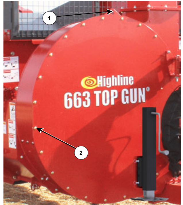
Remove the Blower Front Plate
