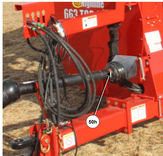
Grease the Over Running Clutch
