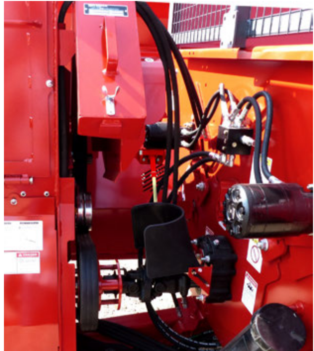
Lift the Blower Drive Shield
