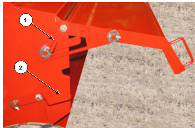
Raise the Auger Housing Cover
