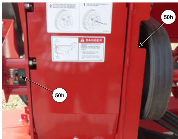
Grease Blower Clutch Shaft (Panel Shown Removed)
