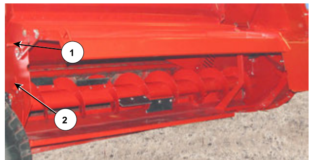
Open the Auger Housing Doors
