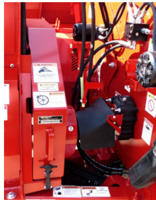
Lower Driveline Shields
