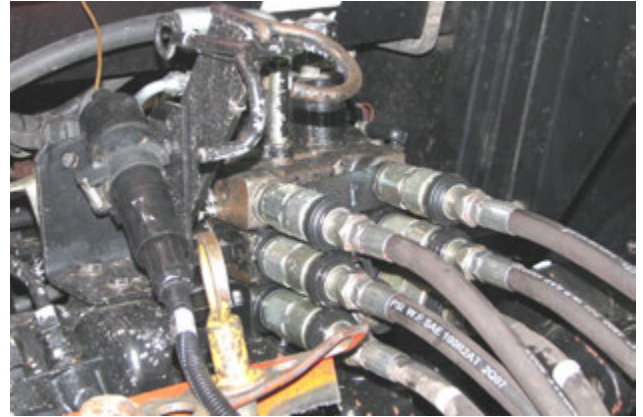
Attach Hydraulics and Electrical (3 Remote Shown)
