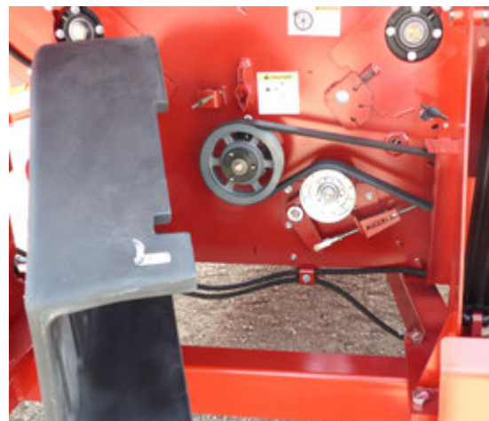
Open the Rear Drive Shield
