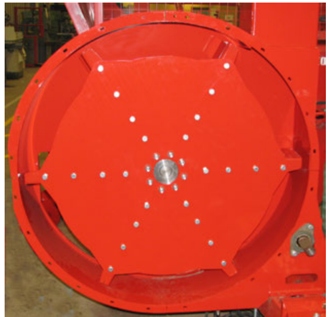
Remove the Front Blower Plate
