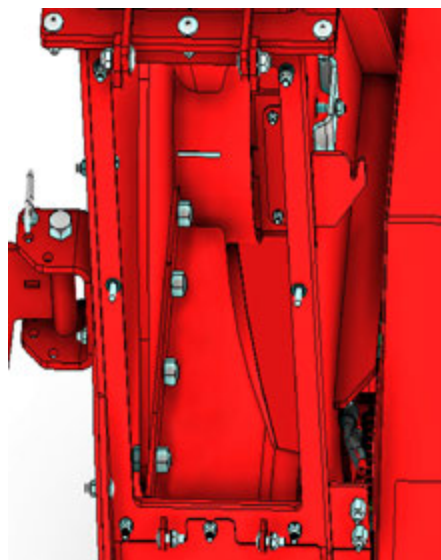
Open Access Panel Clear Blower Housing
