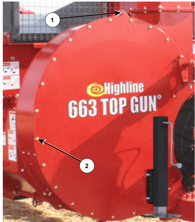
Remove the Blower Front Plate
