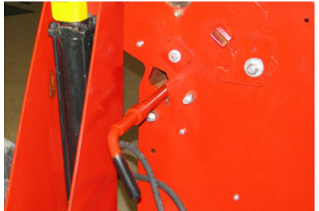
Remove Twine Cutter from Storage Position
