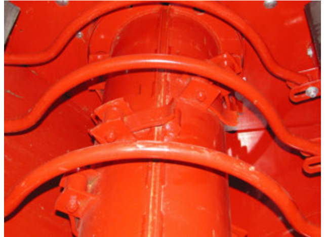
Move Flails Blocking the Knife Path
