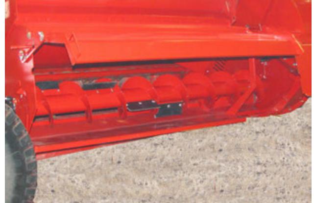
Check Condition of Flighting and Paddles
