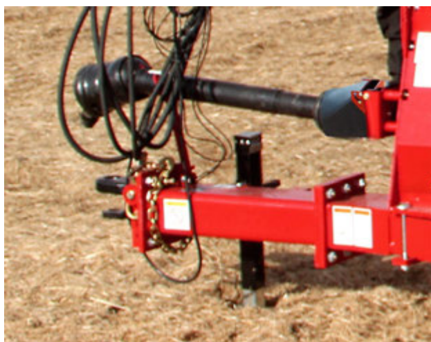
Jack on Hitch - Raise Hitch
