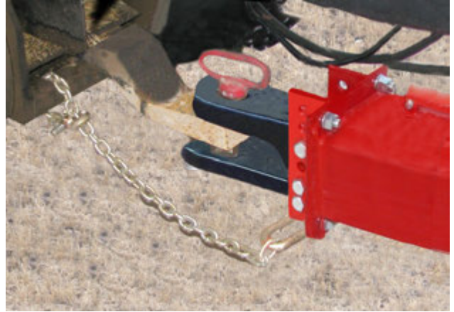
Adjust the Height of Hitch Tongue
