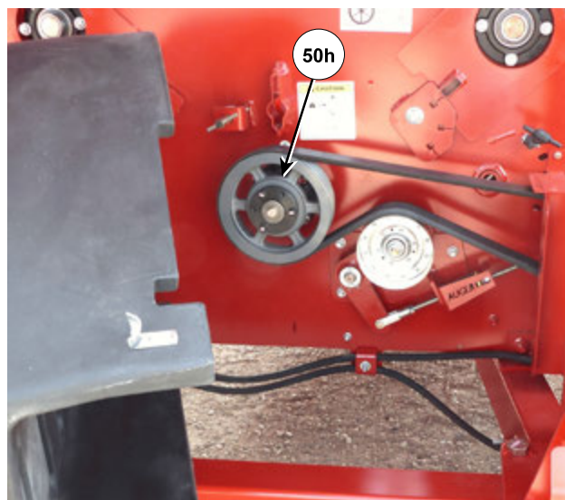
Grease Rear Flail Drum Bearing
