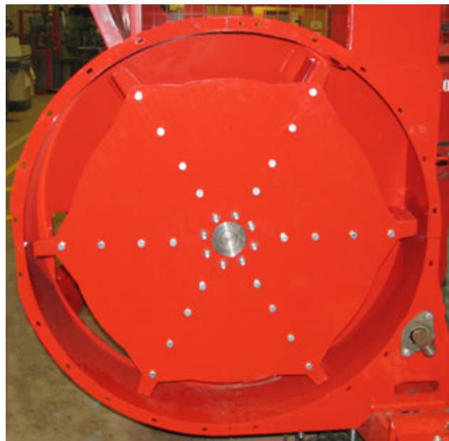
Remove the Front Blower Plate
