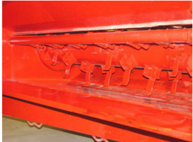
Check Flails (Auger Not Shown for Clarity)
