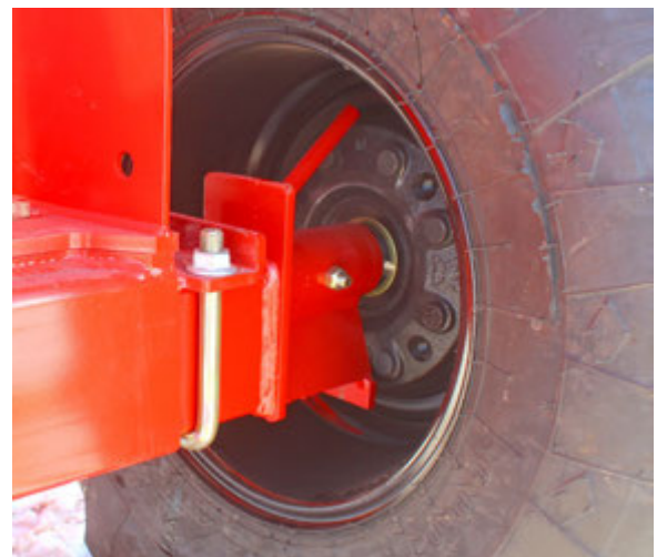
Remove Twine from the Spindle and Hub
