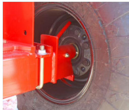
Remove Twine From Spindle and Hub
