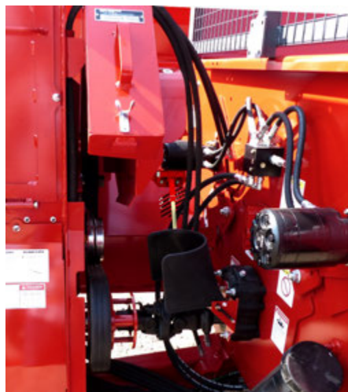
Lift the Drive Shield Check Condition of Drive Belt
