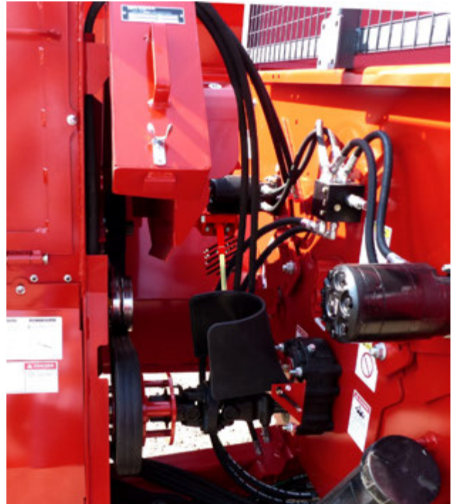
Raise the Blower Drive Shield
