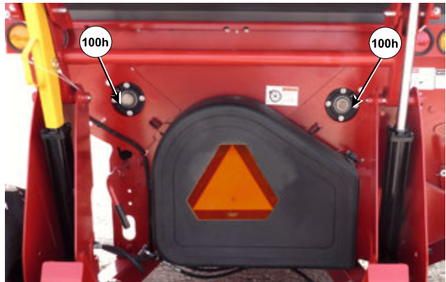
Grease Rear Feed Roller Bearings
