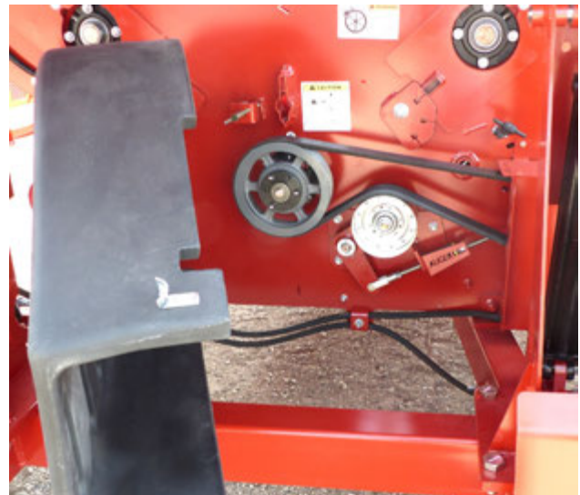
Open the Rear Drive Shield
