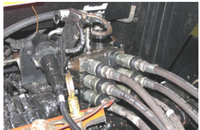
Inspect Hydraulic Hoses (3 Remote Shown)
