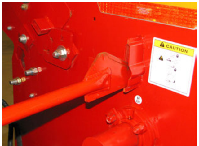
Insert Twine Cutter with Blade Up
