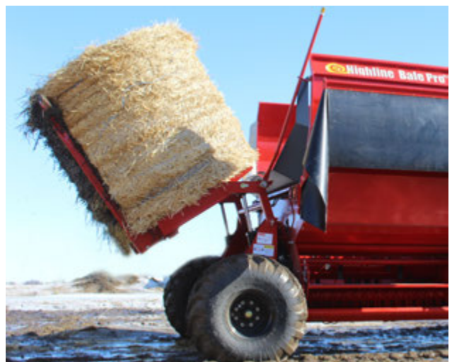
Raise Bale into Processor Tub
