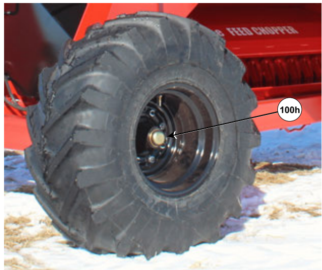
Grease the Hub on Both Spindles
