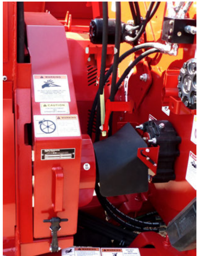
Lower the Drive Shields
