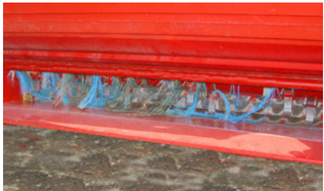
Remove Wrap & Twine (Auger Not Shown for Clarity)
