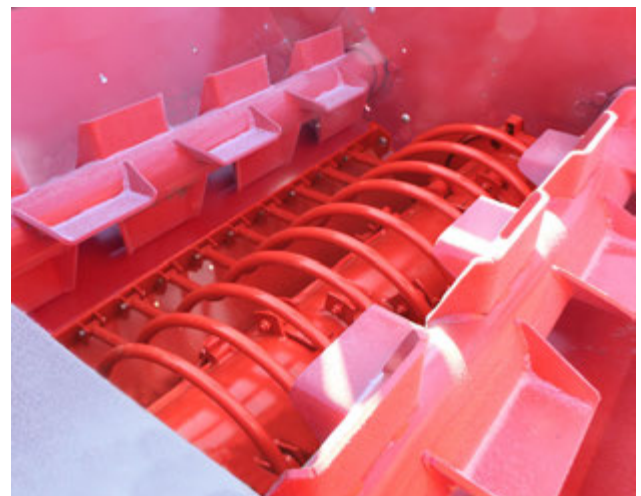
Remove Wrap/Twine from the Feed Rollers
