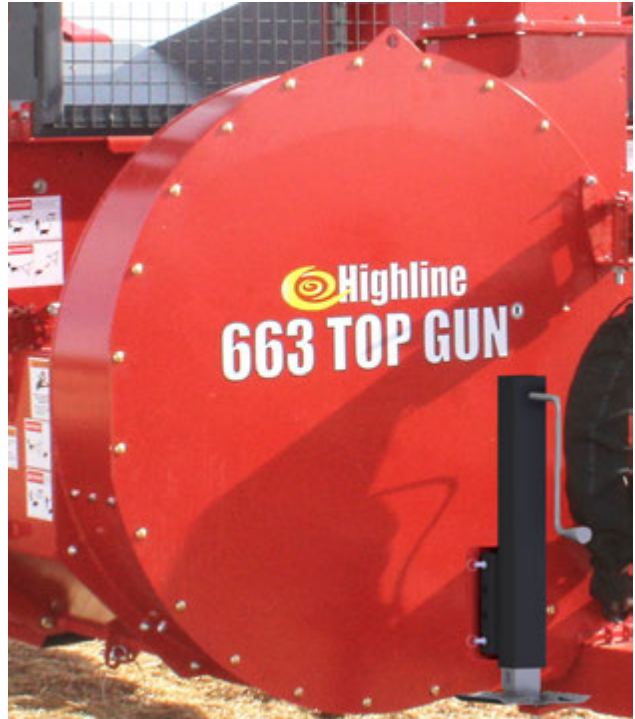
Replace the Front Blower Plate
