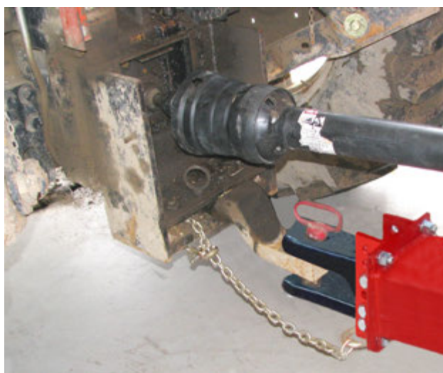
Remove Driveline and Safety Chain
