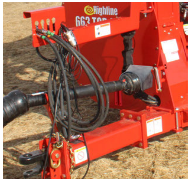
Secure Hoses and Driveline in Supports
