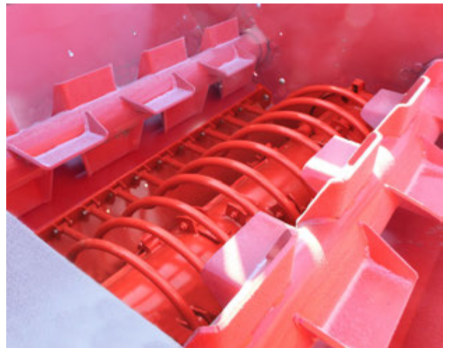
Remove Twine/Wrap from the Feed Rollers
