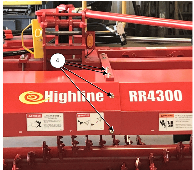
Remove the Fasteners from the Overlap of the Front and Rear Shields 223267C
