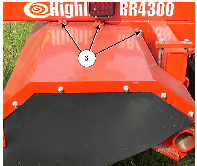
Remove the Rubber Guard Covering the Motor 223256C
