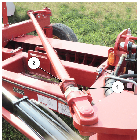
Adjusting the Castor Alignment
