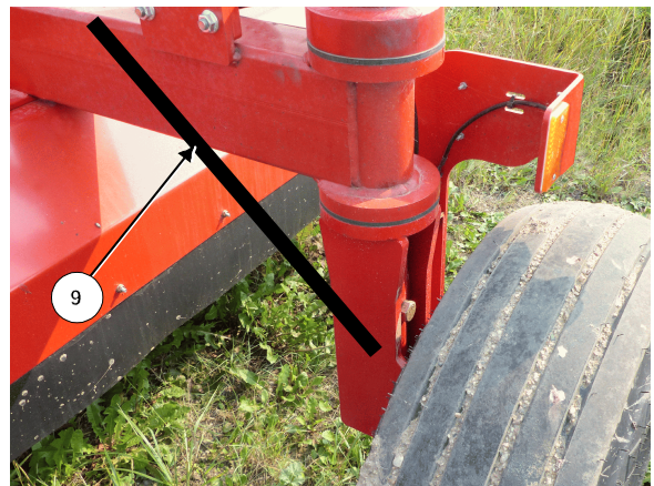
Check Alignment with a Straight Edge
