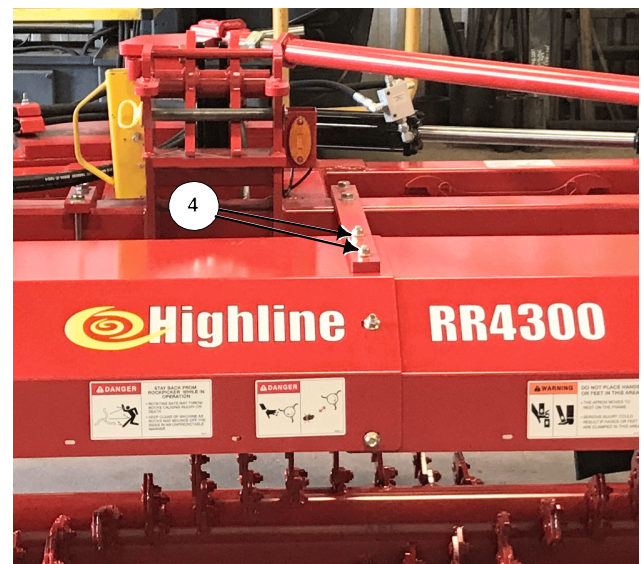
Add Stiffener under the Shield
