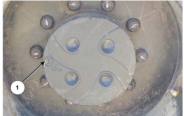
Check Oil Level with Drain Plug Horizontal
