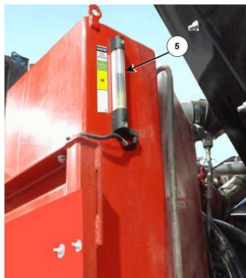
Check the Oil Tank Level
