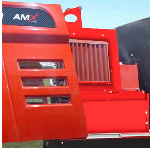
Hydraulic Oil Tank and Cooler
