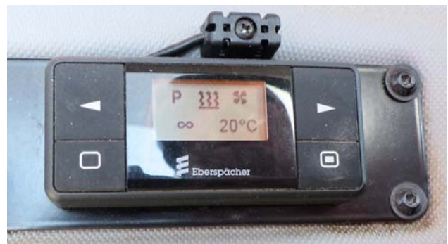
Diesel Heater Control - Cab Heating
