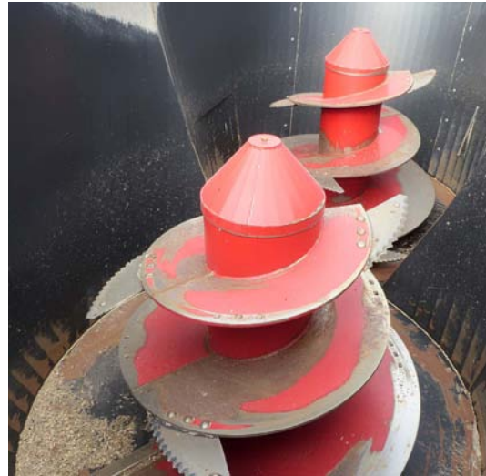
Check for Build Up in the Tub and Condition of the Screws (Optional Knives Shown) 223017
