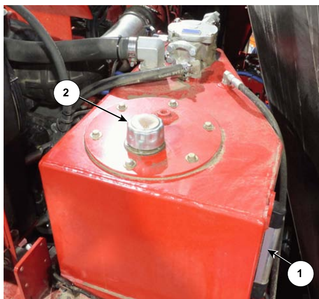
Oil Tank Level and Fill
