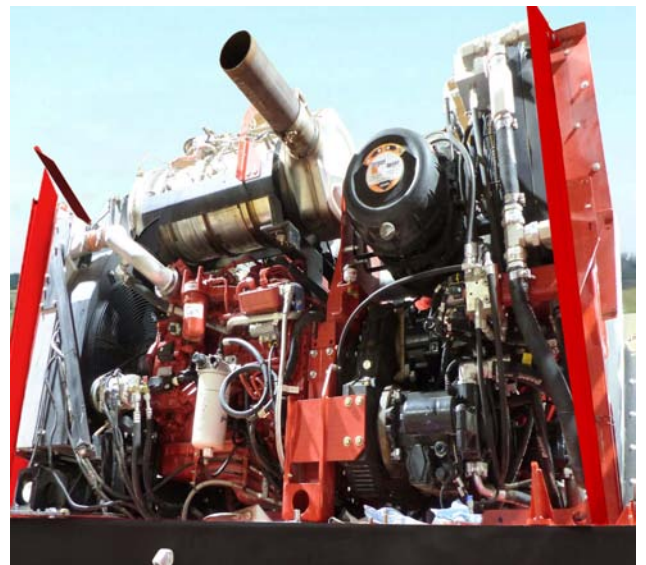
Engine and Hydraulic Pumps
