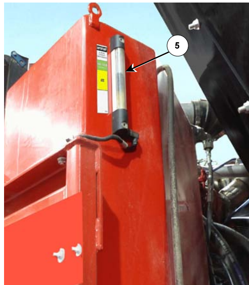
Check the Oil Tank Level
