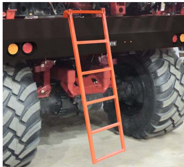
Use Ladder to Access Engine and Pumps
