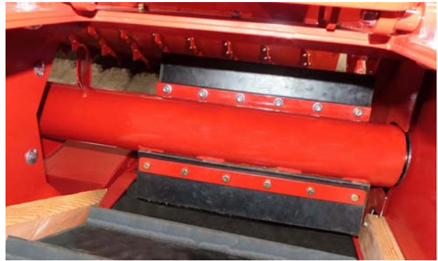
Clear Plugging from Auger Area
