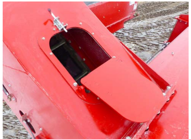
Lift Mineral Loading Door for Access to Auger and Loading Paddles 220071
