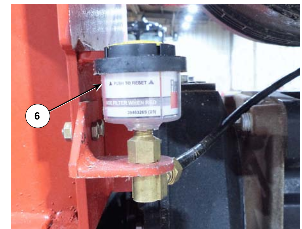
Push to Reset Air Indicator - Red Band Gone
