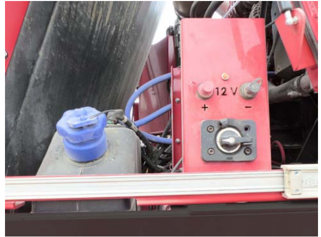
DEF Tank Location
