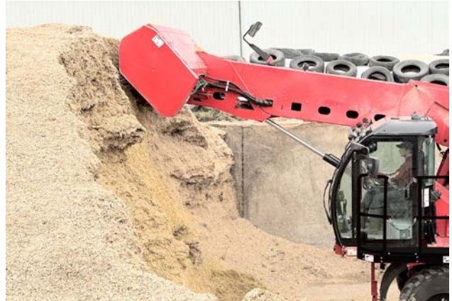
Raise Milling Arm to Top of the Pile
