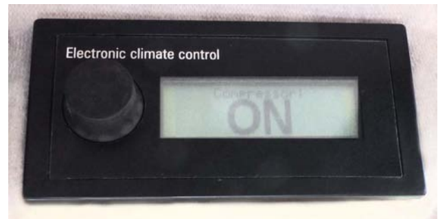
Air Conditioning Control - Cab Cooling
