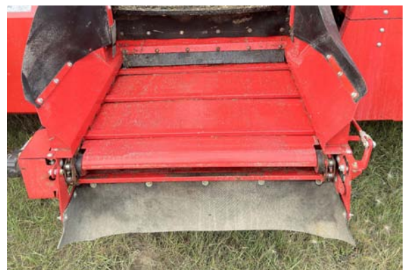
Start the Unload Conveyor
