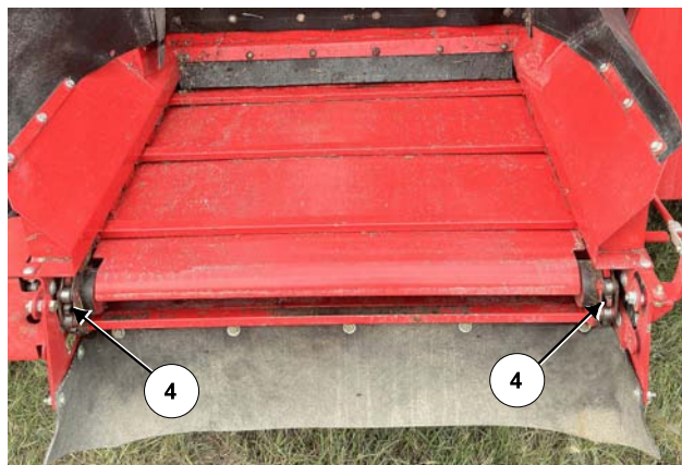
Clean the Front Teeth of the Conveyors
