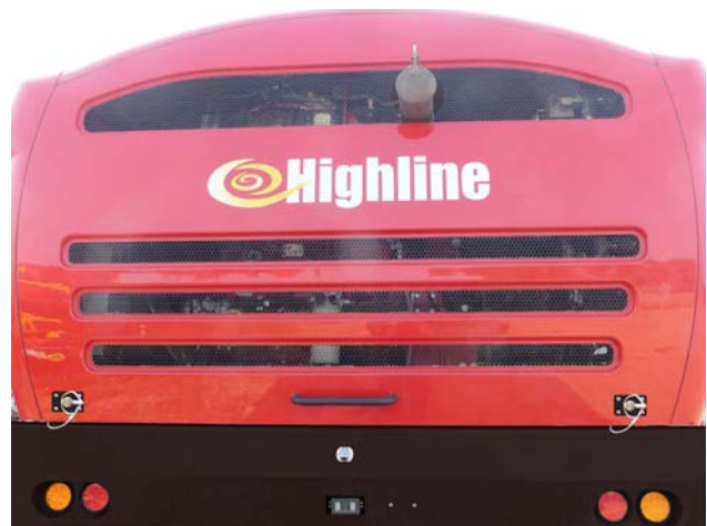
Clean Rear Screens
