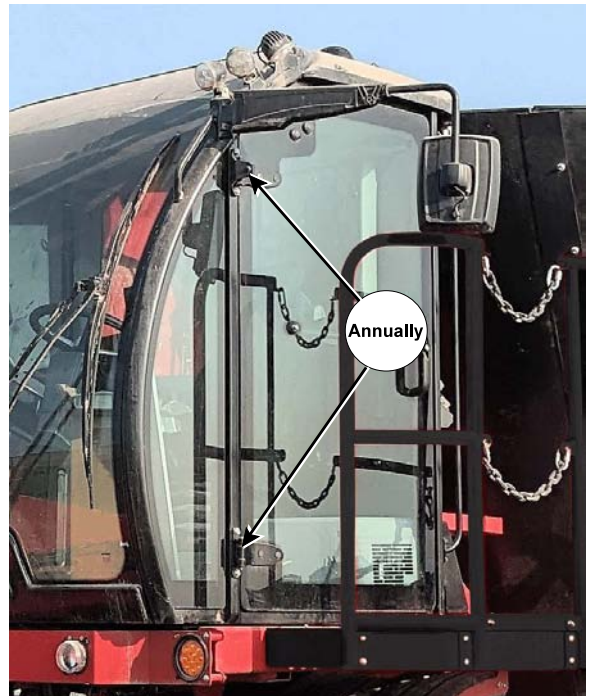
Grease the Cab Door Hinges
