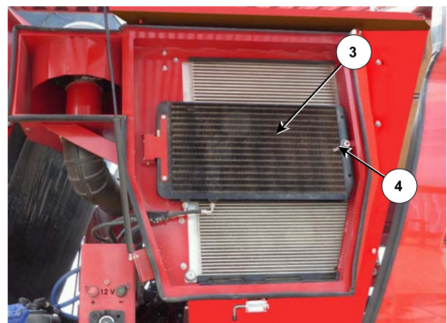
Clean Inner Radiator and Screens
