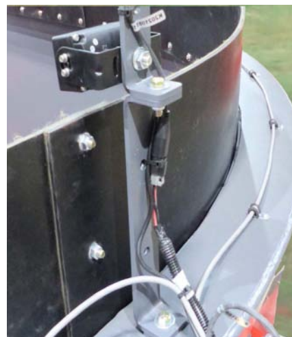
Attach Cables to Top of Tank Rim
