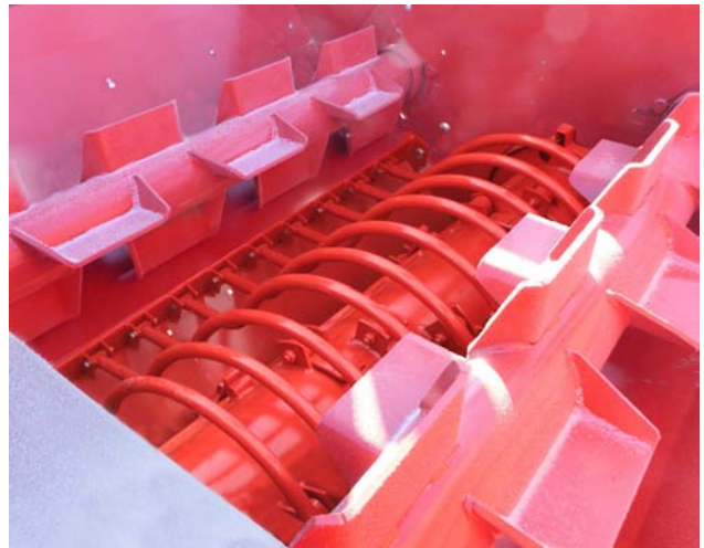
Remove Twine/Wrap from the Feed Rollers
