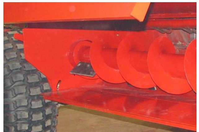
Remove Twine From Auger
