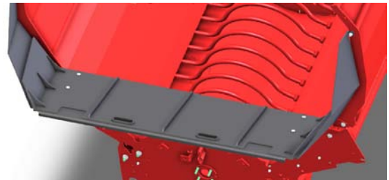
Adjust the Rear Deflector Shield (Deflector Shown Pushed in for Round Bales) 222035
