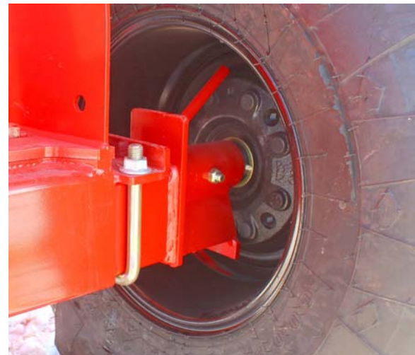
Remove Twine from the Spindle and Hub
