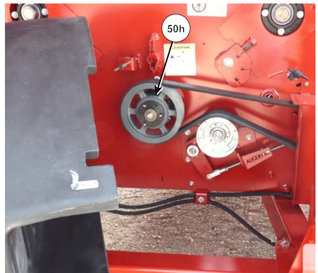
Grease Rear Flail Drum Bearing
