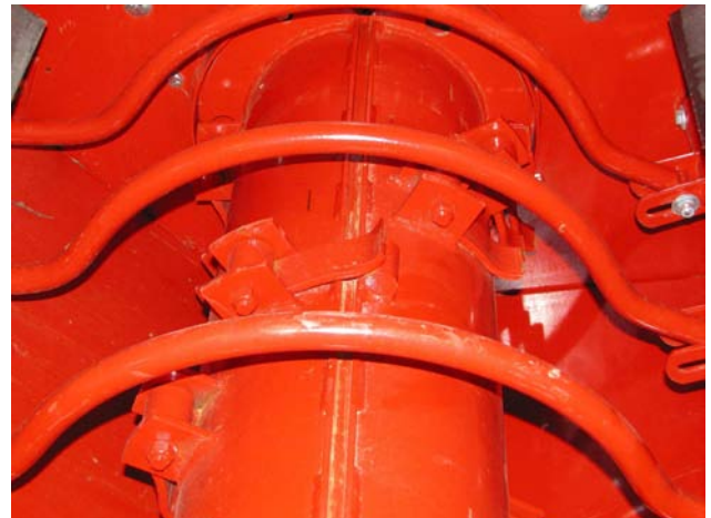
Move Flails Blocking the Knife Path
