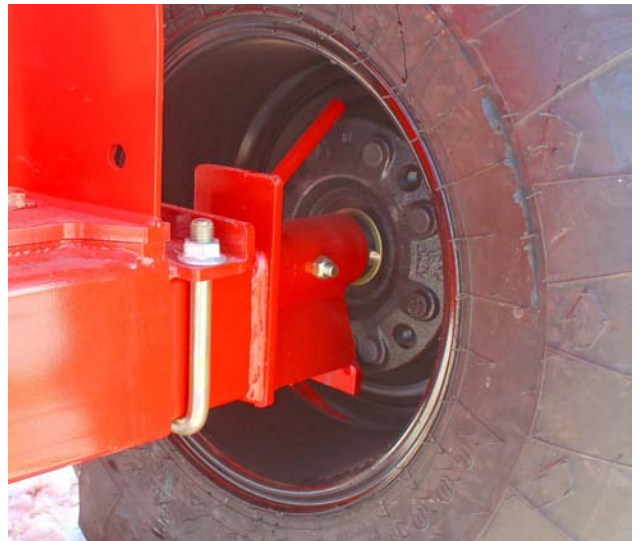
Remove Twine From the Spindle and Hub
