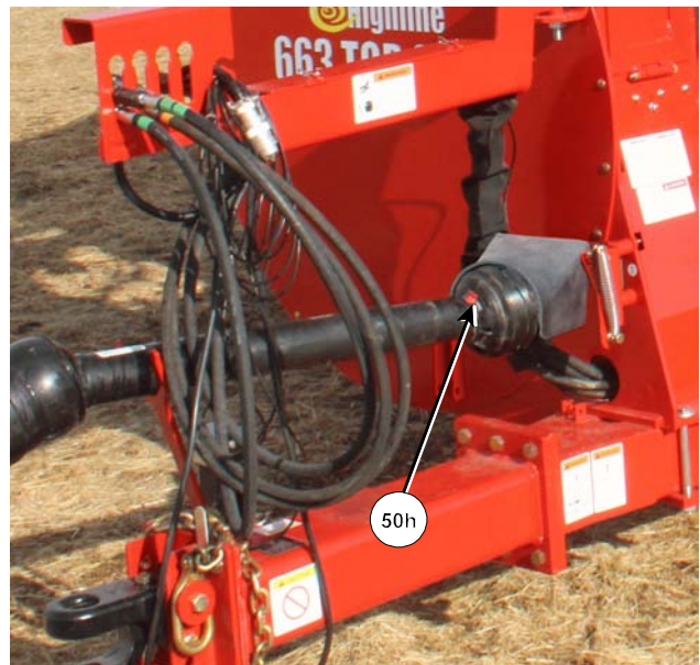
Grease the Over Running Clutch
