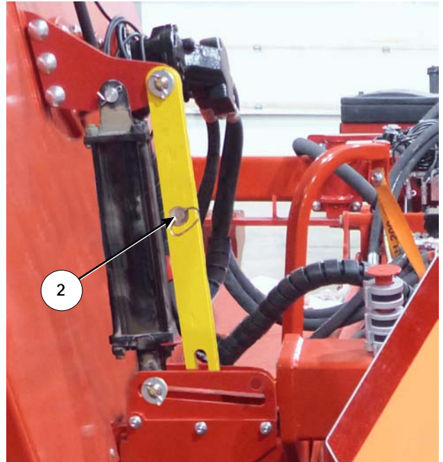
Remove Wing Transport Lock Pins Place Pins in Storage Positions
