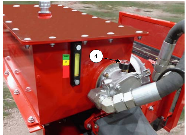
Check Oil Filter Operating Pressure
