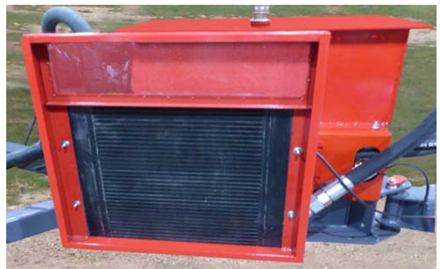
Clear Debris from Oil cooler
