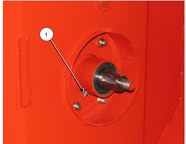
Grease Blade Hub (Pan Shown Removed for Clarity) 214059C
