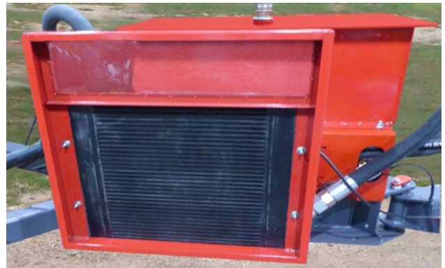
Clear Debris from Oil cooler
