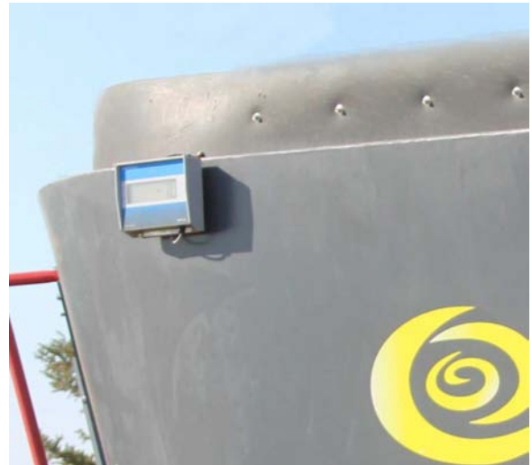
Remote Display Mounted on Tub Wall (Left Side Shown)
