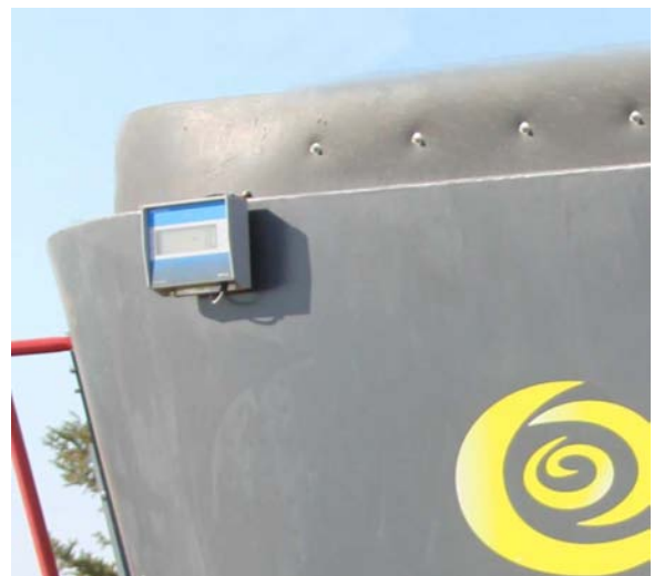
Remote Display Mounted on Tub Wall (Left Hand Side Shown)
