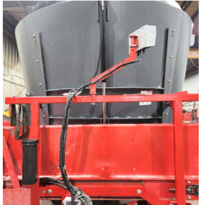
Route the cables (Front center mounting location shown)
