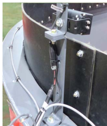
Attach Cables to Top of Tank Rim
