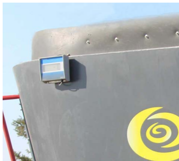
Remote Display Mounted on Tub Wall
