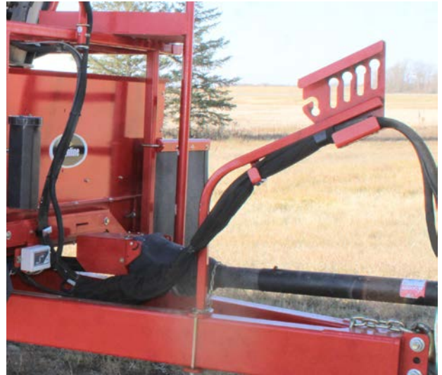
Figure 17: Route the Hoses Through the Abrasion Sleeve and Into the Hose Holder 222310
