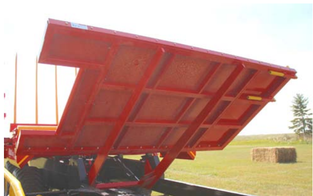
Check The Front Table Raises and Lowers
