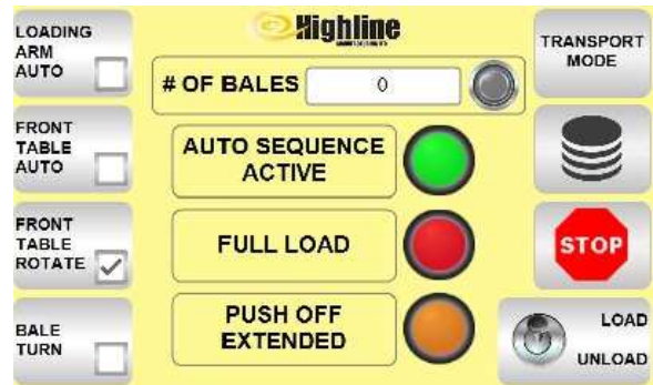
Push Front Table Rotate Button
