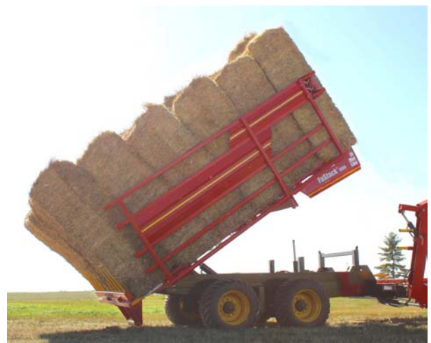
Raise Table, Let Bales Slide, Open Side Rails
