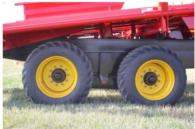
Jack Under Spindle Tube to Change Tire
