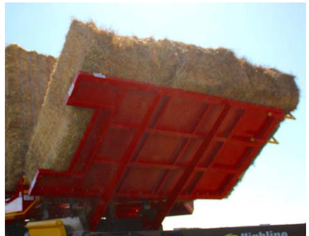
Press Front Table Up - Raise Front Table
