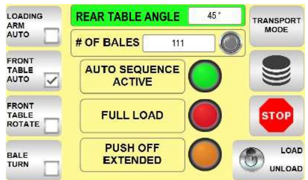
Rear Table Angle Readout
