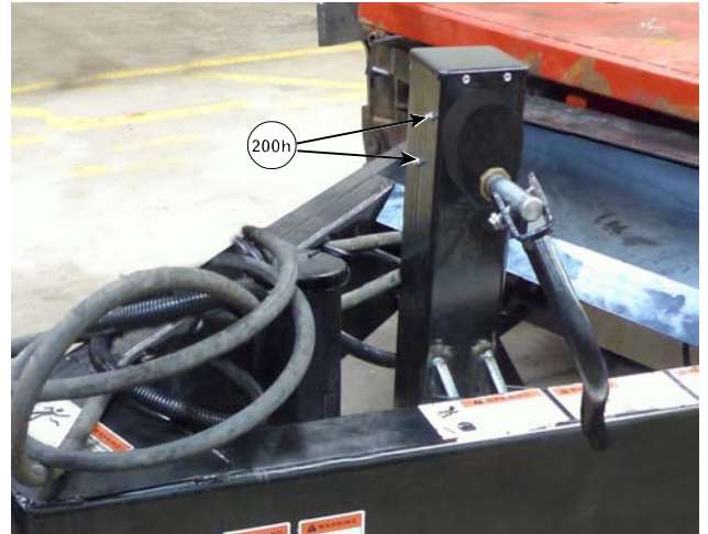
Grease the Hitch Jack
