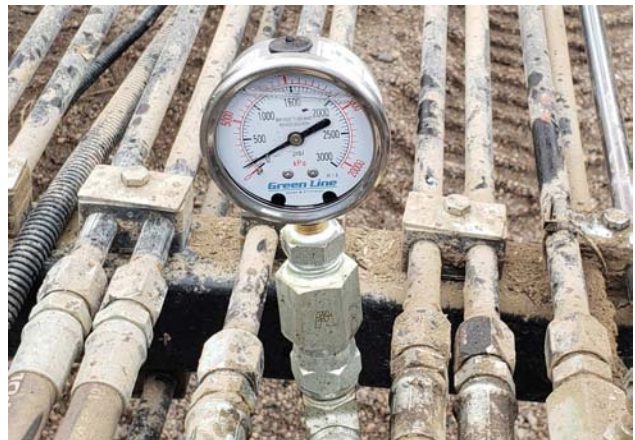
Trace the Hydraulic Line with the Pressure Gauge to the Valve
