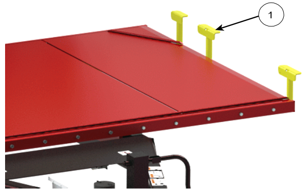
Adjust Front Table Stops
