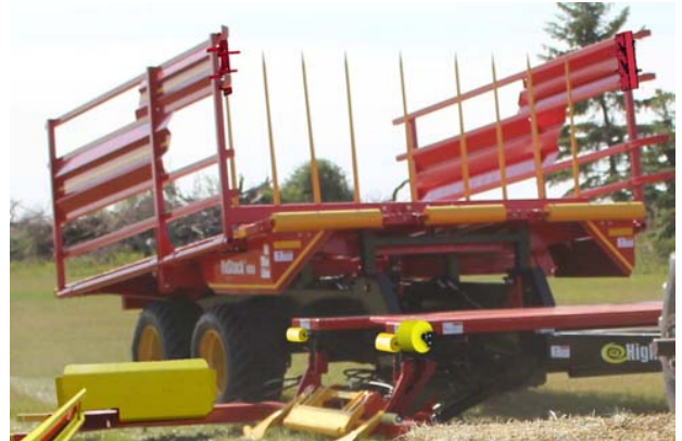
Lower Front Table ,Lower Lift Arm
