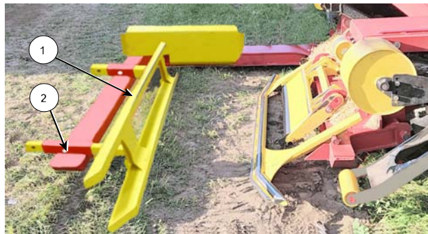
Adjust Arm for 3 Foot (0.9 m) Bales
