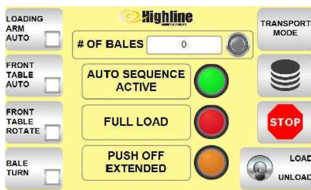
Select Unload on the Display
