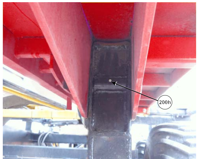
Grease Rear Table Pivots (Right Side Shown)
