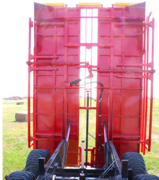
Check The Rear Table Raises and Lowers
