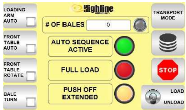
Push Off Extended Warning Light
