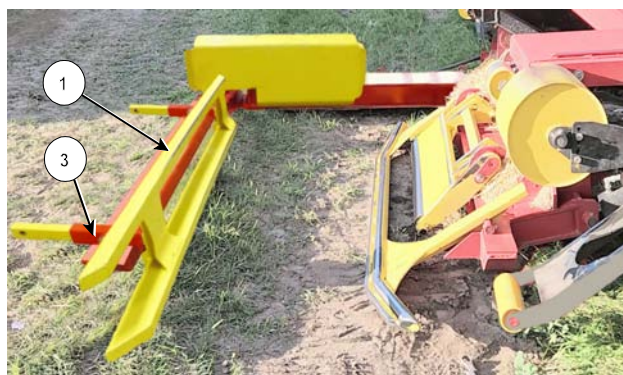
Adjust Arm for 4 Foot (1.2 m) Bales
