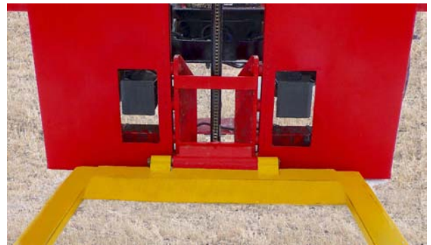
FaStack 1200 Retract Push Off Cylinders
