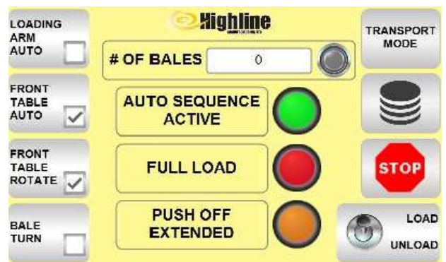
Front Table Auto with Table Rotate
