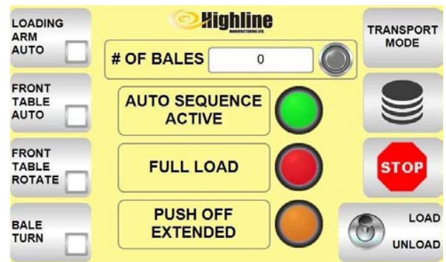
Front Table Rotate Turned Off
