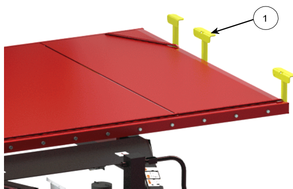
Adjust Front Table Stops
