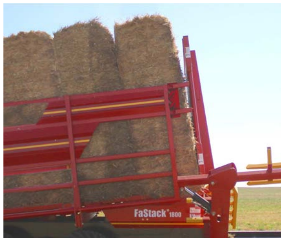
Fully Raise Front Table, Close Side Racks
