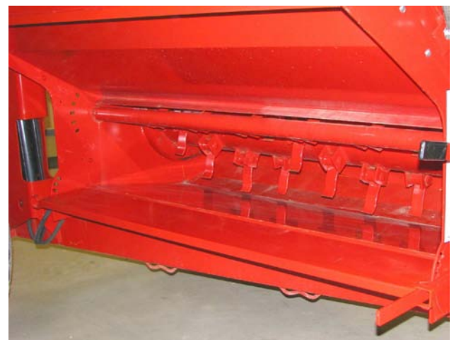
Check and Clean Flail Drum Area (Auger Not Shown for Clarity)
