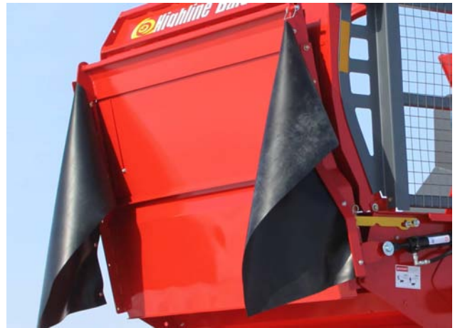
Discharge Door Raised - Rubber Secured
