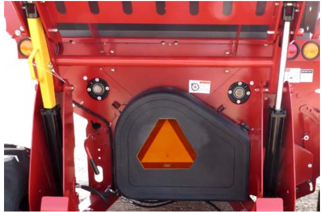
Close the Rear Drive Shield
