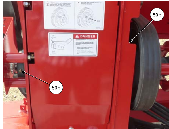
Grease Blower Clutch Shaft (Panel Shown Removed)
