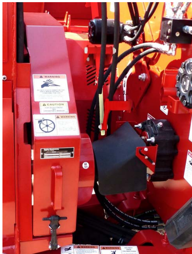
Lower the Drive Shields
