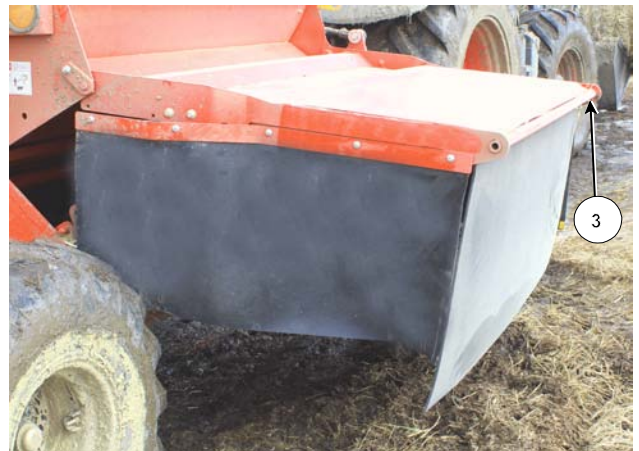
Set the Upper Deflector Door (Bunk or Windrowing Shown)
