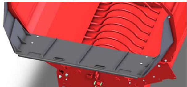
Adjust the Rear Deflector Shield (Deflector Shown Pushed in for Round Bales)
