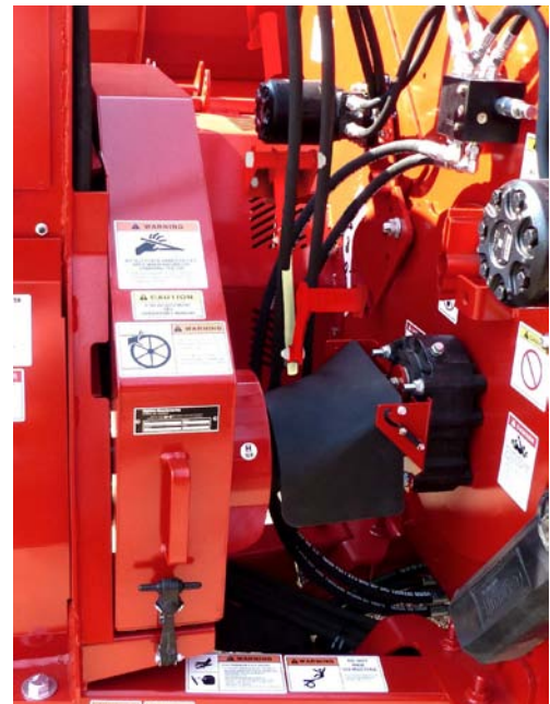
Lower Driveline Shields
