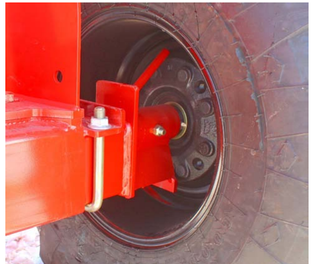
Remove Twine from the Spindle and Hub
