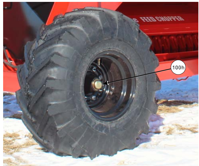
Grease the Hub on Both Spindles
