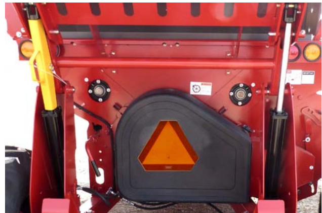
Close the Rear Drive Shield
