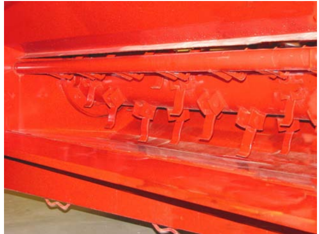
Check Flails (Auger Not Shown for Clarity)
