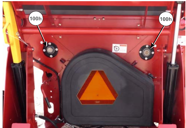
Grease Rear Feed Roller Bearings
