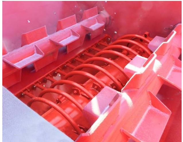
Remove Twine/Wrap from the Feed Rollers
