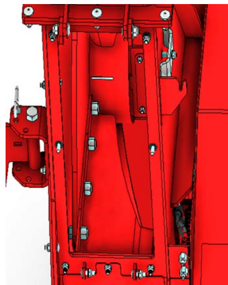
Open Access Panel Clear Blower Housing
