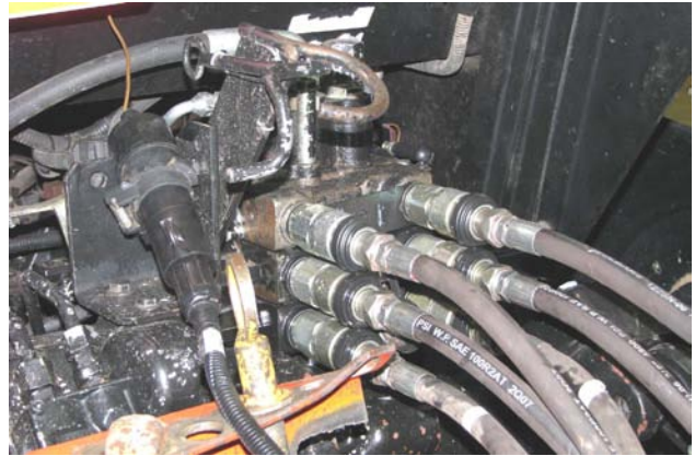
Disconnect Hydraulic Hoses & Electrical
