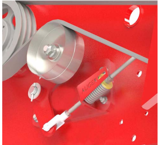
Check the Auger Belt and Tension
