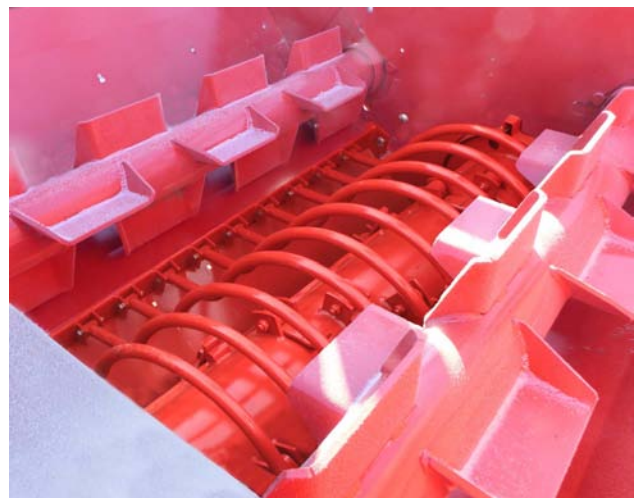
Remove Wrap/Twine from the Feed Rollers
