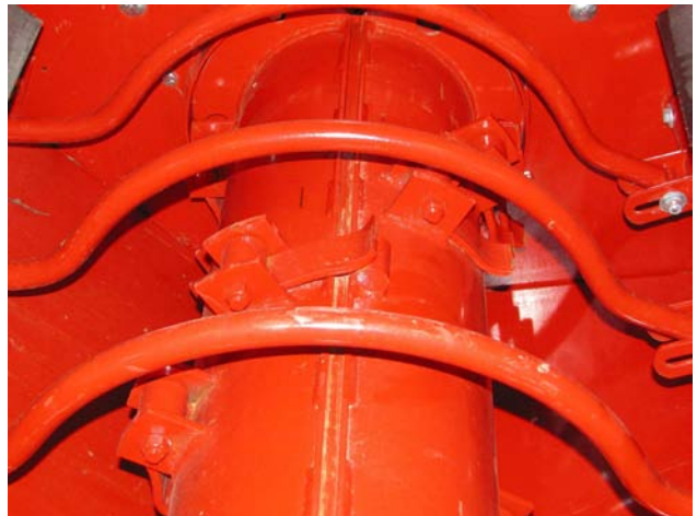
Move Flails Blocking the Knife Path
