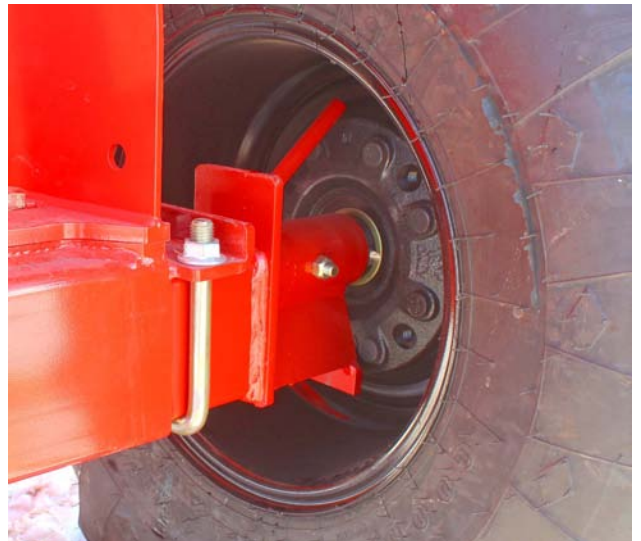
Remove Twine From the Spindle and Hub
