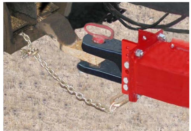
Adjust the Height of Hitch Tongue
