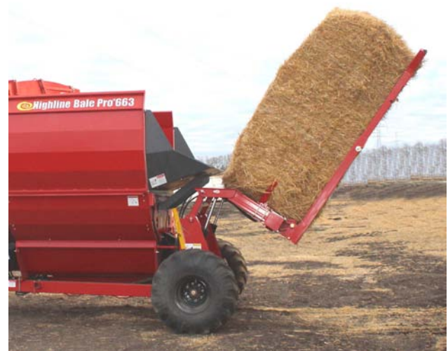
Shut Down Flail Drum When Loading Tub
