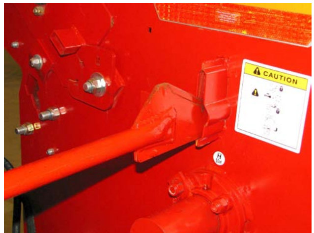
Insert Twine Cutter with Blade Up
