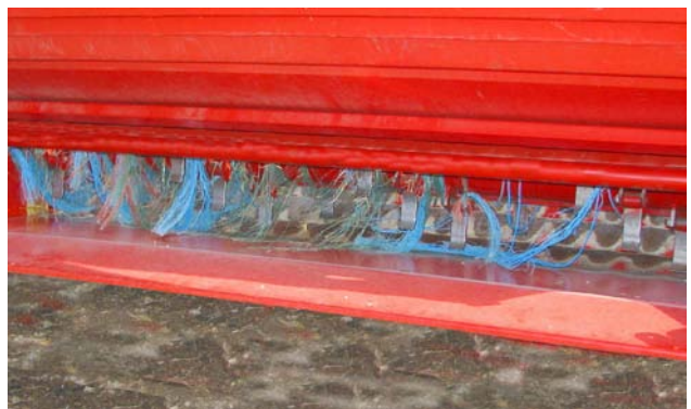
Remove Wrap & Twine (Auger Not Shown for Clarity)
