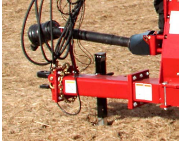
Lift Hitch with the Jack
