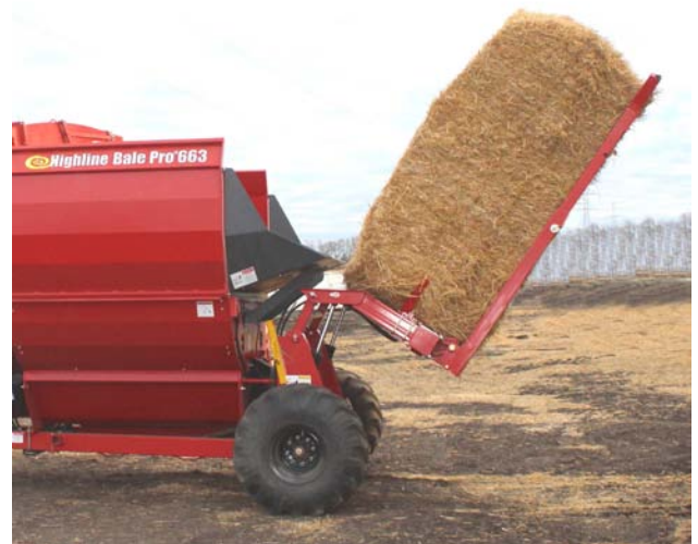
Raise Bale into Processor Tub
