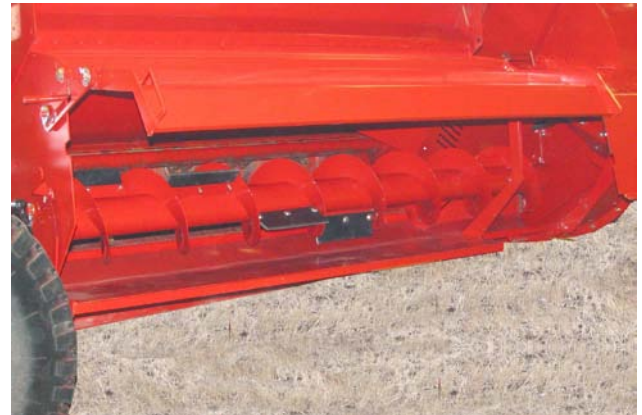
Check Condition of Flighting and Paddles
