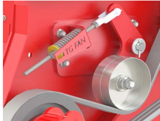
Check Blower Drive Belt and Tension
