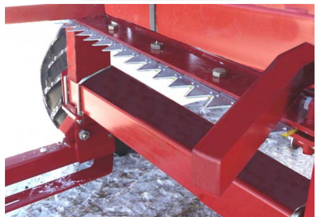
Check the Twine Sickle Moves
