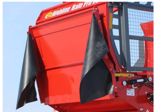
Discharge Door Raised - Rubber Secured
