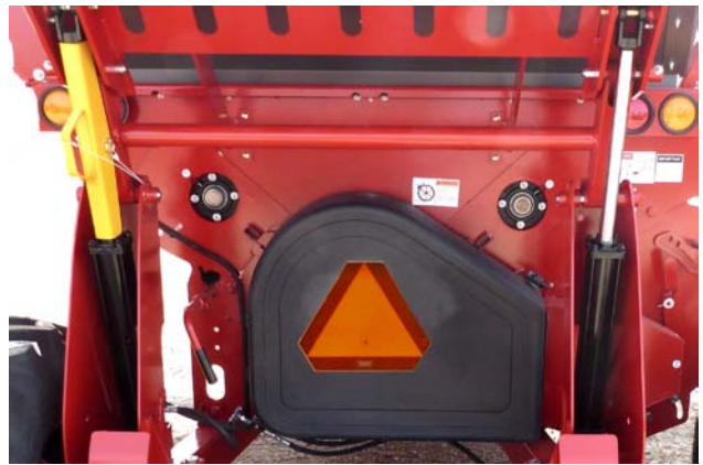
Close the Rear Drive Shield
