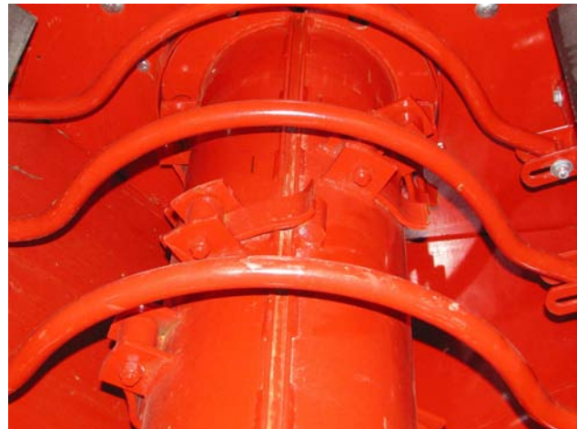
Move Flails Blocking the Knife Path
