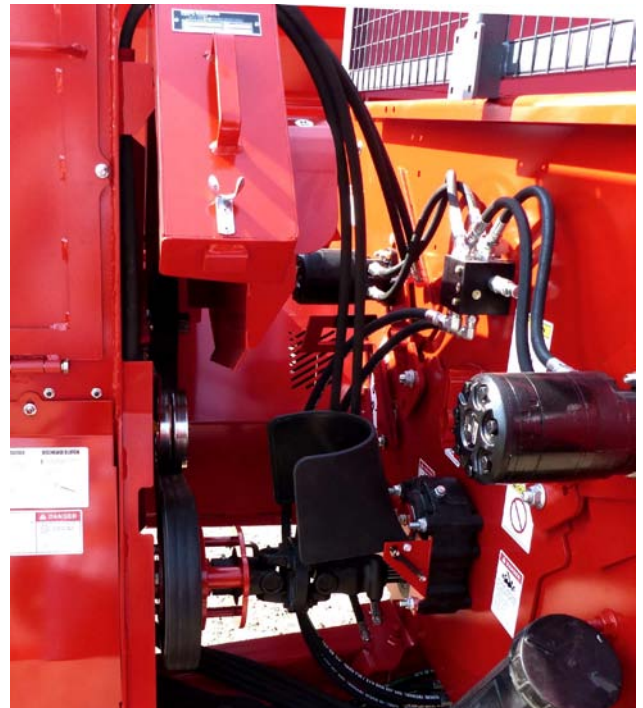
Lift the Drive Shield
