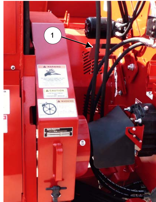
Move Flail Guard Rod Lever
