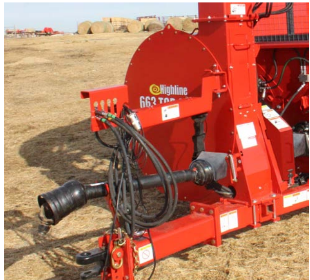
Hoses and Driveline in Supports
