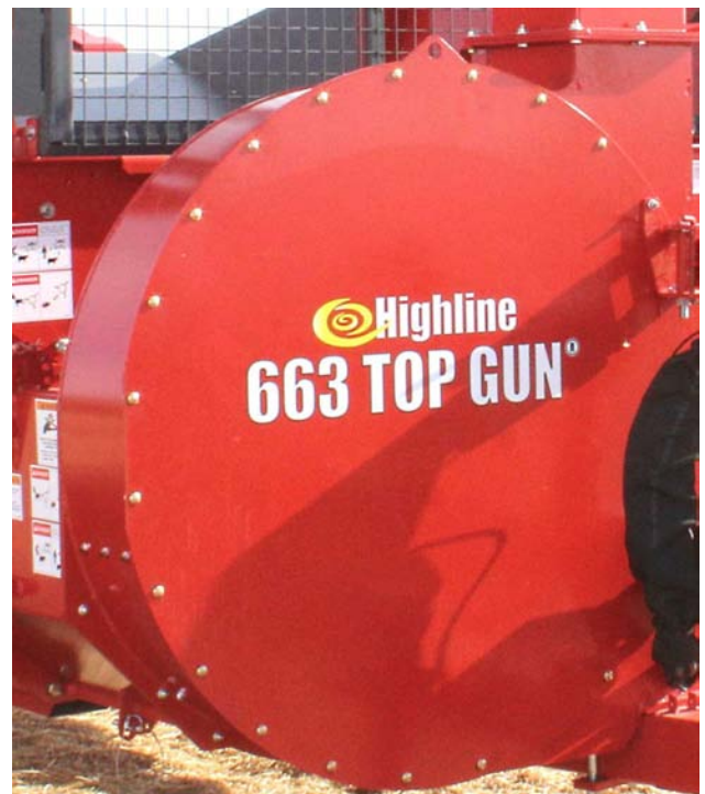
Replace the Front Blower Plate
