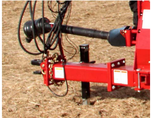
Lift Hitch with the Jack
