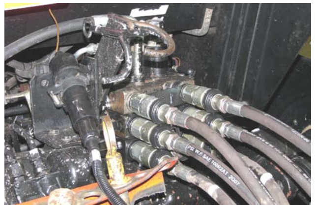
Inspect Hydraulic Hoses
