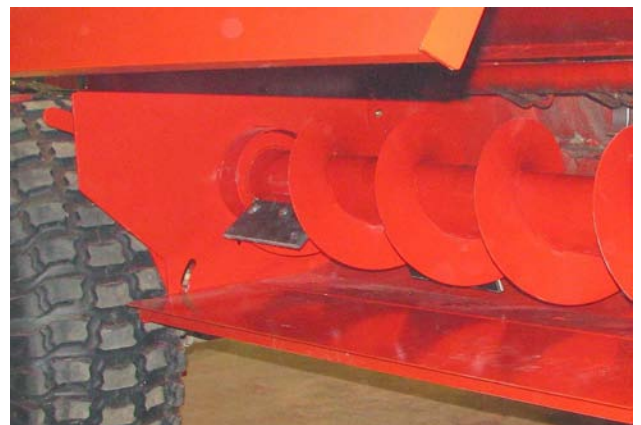
Remove Twine From Auger
