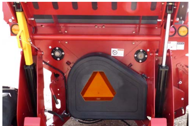
Close the Rear Drive Shield
