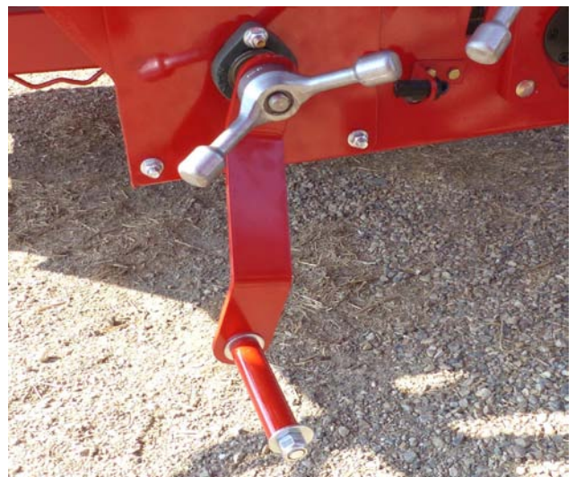
Hand Crank Attached to Auger Flighting
