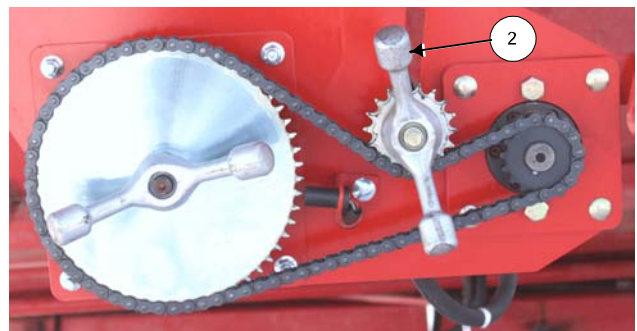
Loosen and Remove the Drive Chain
