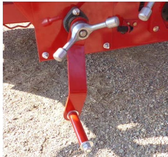
Hand Crank Onto Auger Shaft
