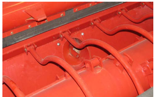
Clear Auger Discharge Inside Tub
