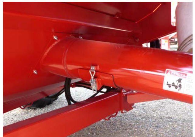
Close the Auger Calibration Cover
