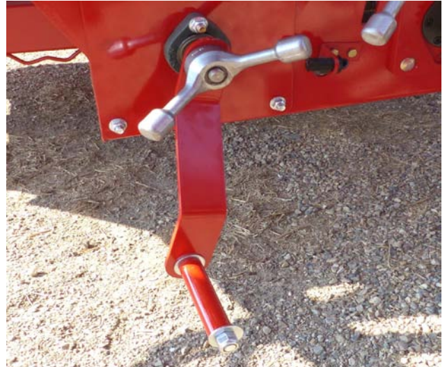
Hand Crank Attached to Auger Flighting
