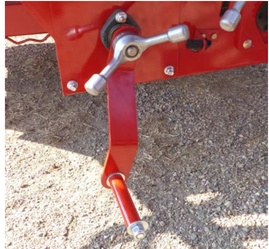
Rotate Auger to Remove Product
