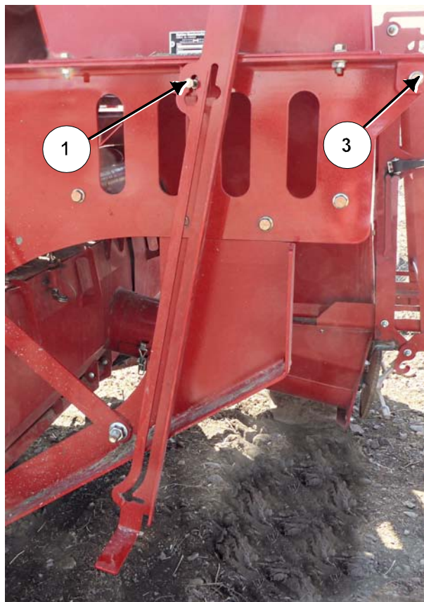
Move the Lid Handle into the Storage Position
