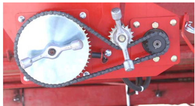
Lubricate the Auger Drive Chain
