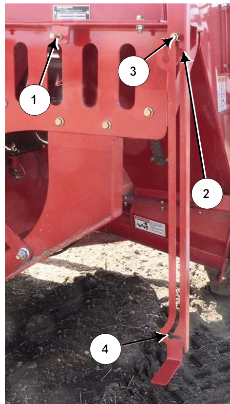
Move the Lid Handle into the Lifting Position
