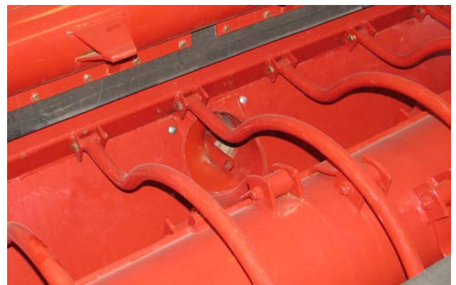
Clear Auger Discharge Inside Tub
