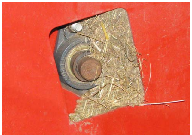
Remove Material - Lower Chain Bearing
