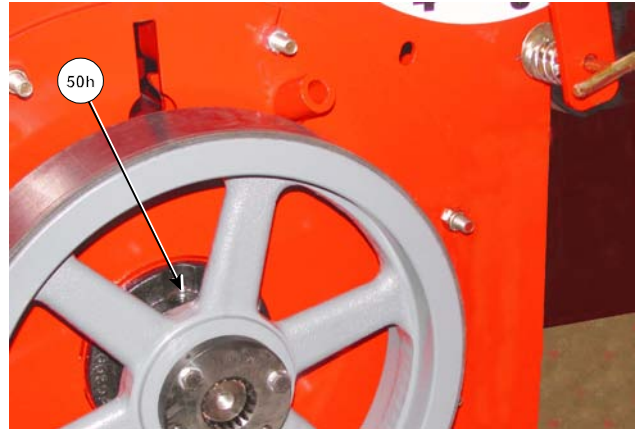
Lubricate the Driveline Sheave Bearing (Drive Shield Not Shown for Clarity)
