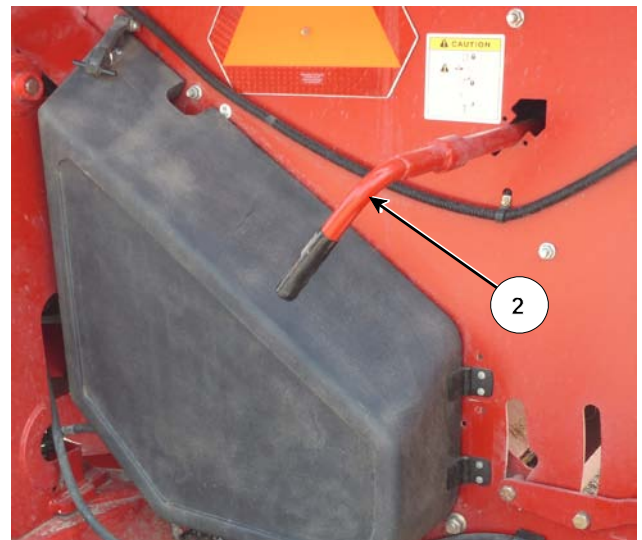
Remove Twine Cutter from Storage
