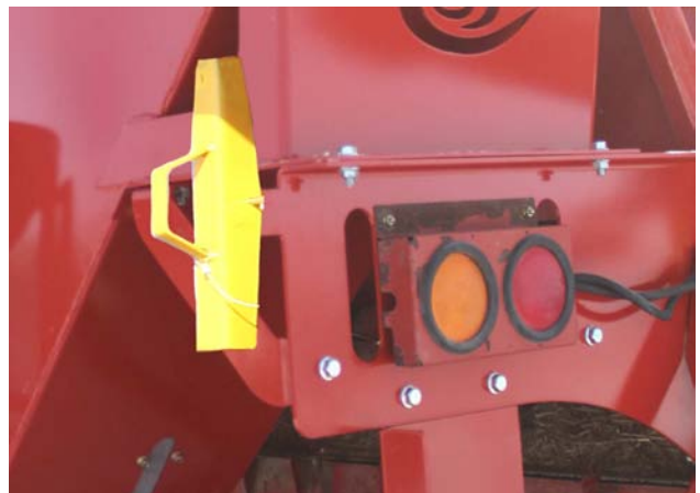
Cylinder Lock Stored (With Grain Tank) 221323
