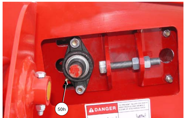
Grease Upper Feeder Chain Bearings
