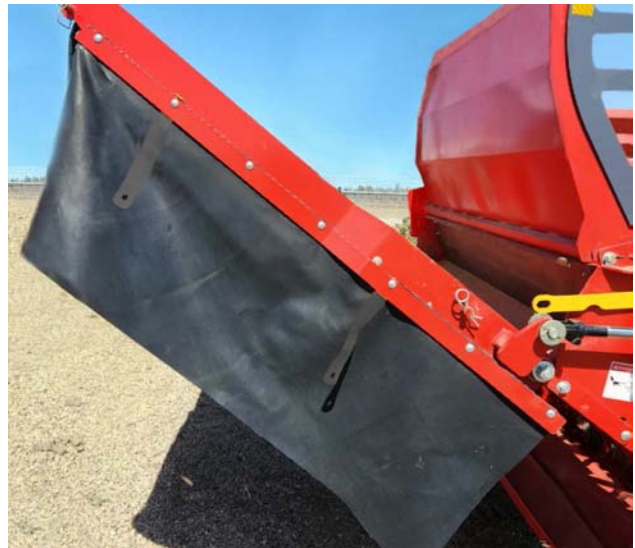
Side Curtains Loosened for Bunk or Windrow
