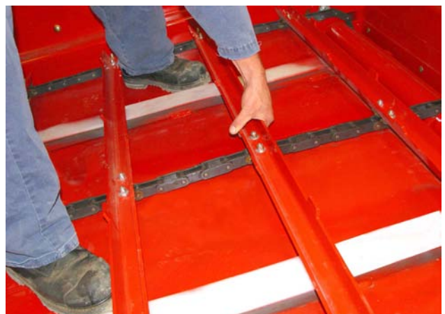
Check Tension of the Feeder Chain
