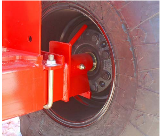
Remove Twine from the Spindle and Hub
