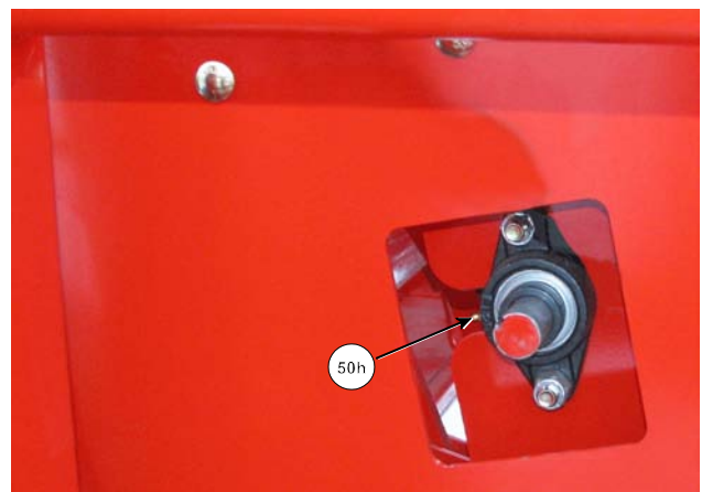
Grease Rear Lower Feeder Chain Bearing
