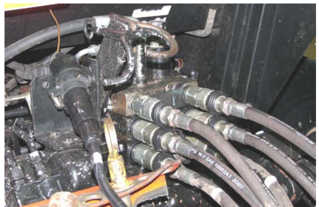
Disconnect Hydraulic Hoses & Electrical
