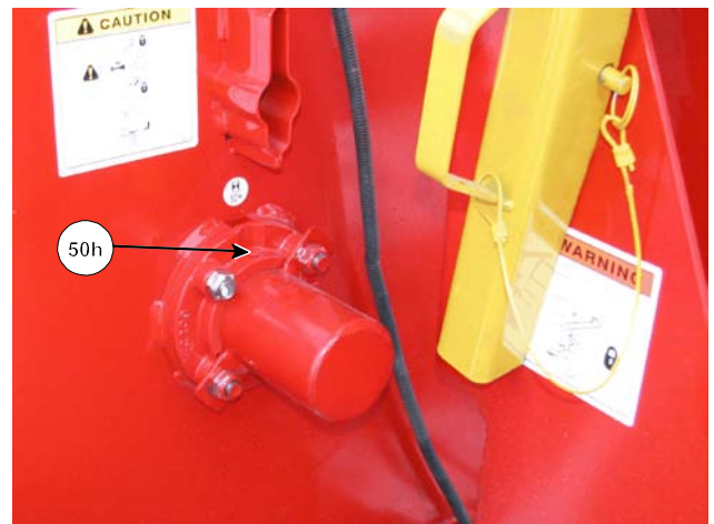
Grease Rear Flail Drum Bearing
