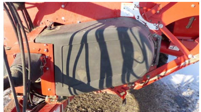
Ensure Driveline Shields are in Place
