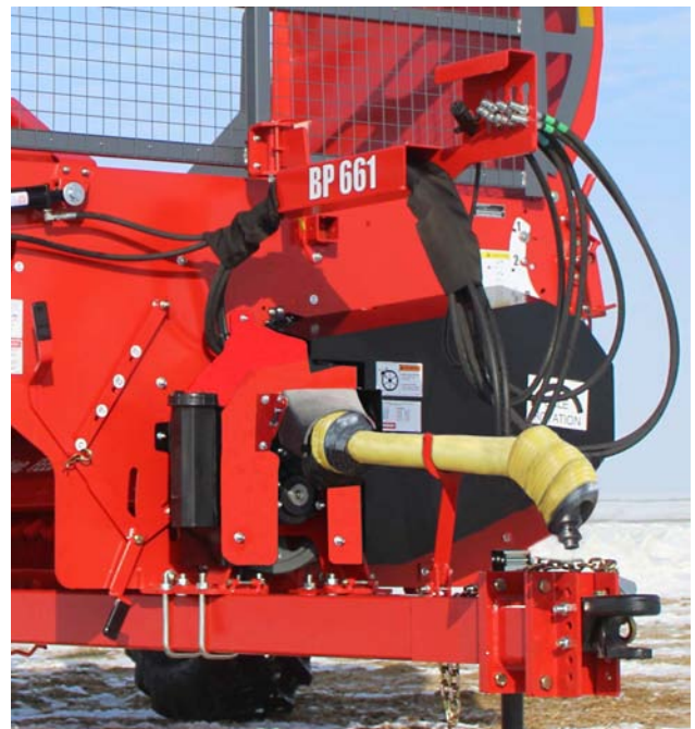
Rest the Driveline in the Drive Holder
