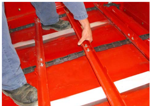
Check Tension of the Feeder Chain
