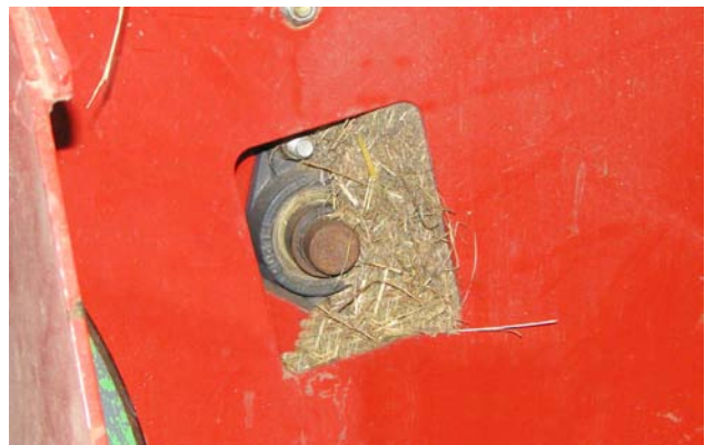
Remove Material - Lower Chain Bearing
