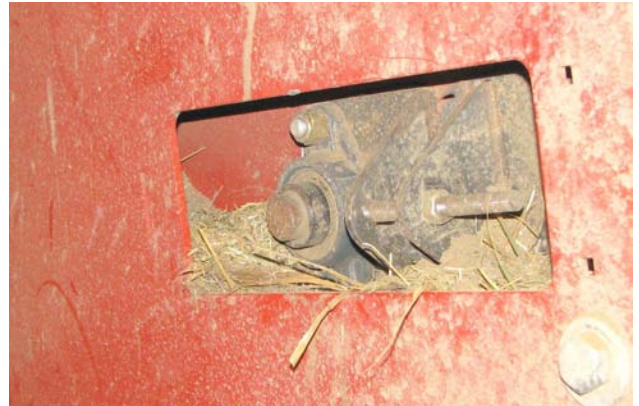
Remove Material - Upper Chain Bearing
