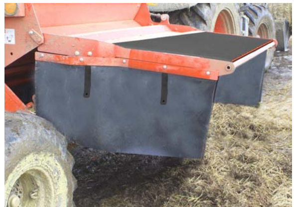
Rubber On Top of Door for Bedding
