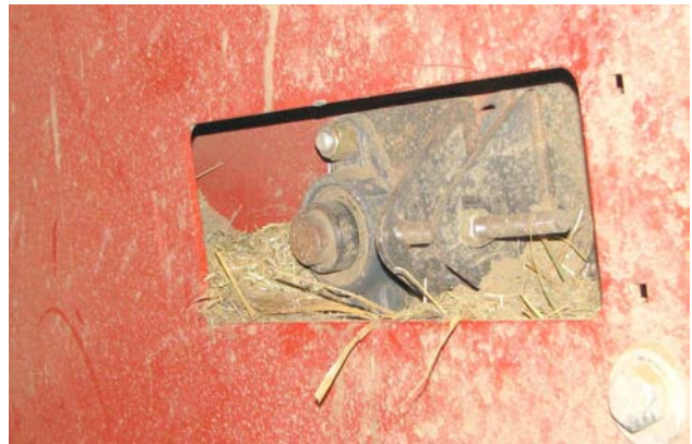
Remove Material - Upper Chain Bearing
