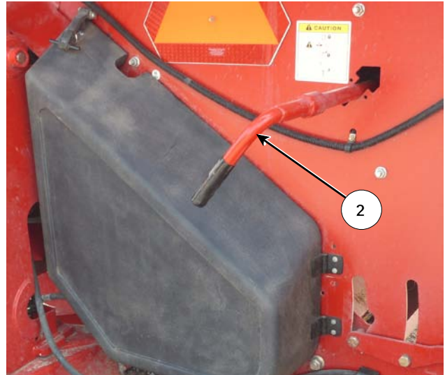
Replace Twine Cutter Into Storage Position
