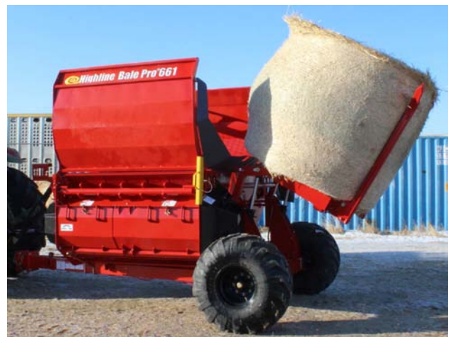
Raise Bale into Processor Tub
