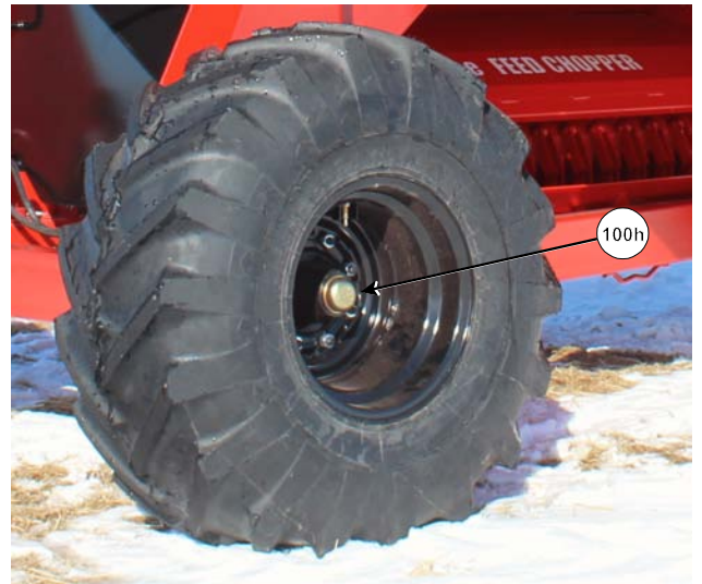
Grease Hubs on Both Spindles
