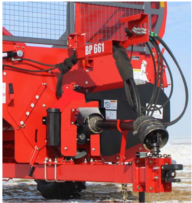
Hoses and Driveline in Supports
