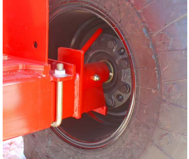
Remove Twine From the Spindle and Hub
