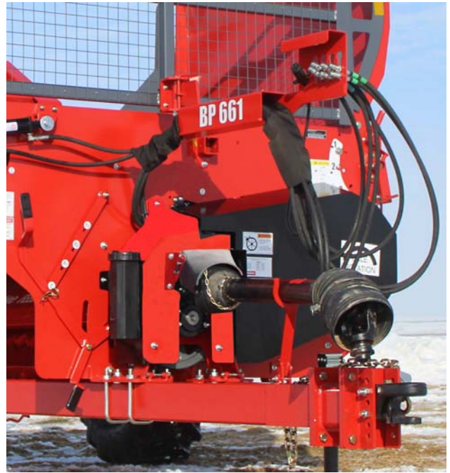
Hoses and Driveline in Supports
