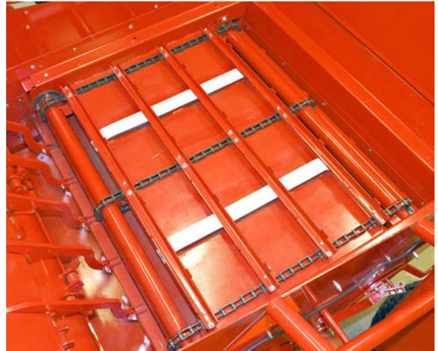
Check Condition of Feeder Chain
