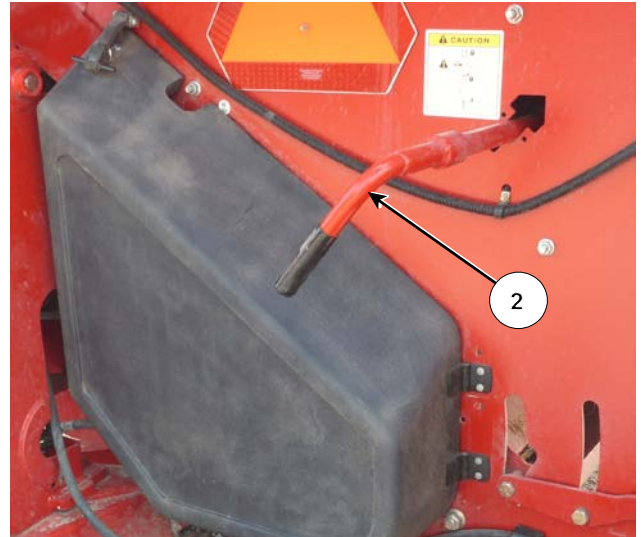
Replace Twine Cutter Into Storage Position
