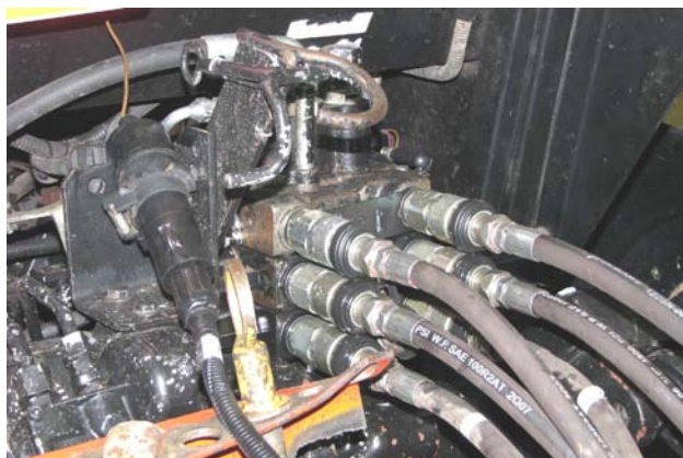
Attach Hydraulics and Electrical
