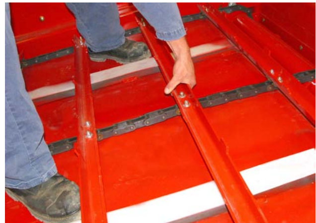
Check Tension of the Feeder Chain
