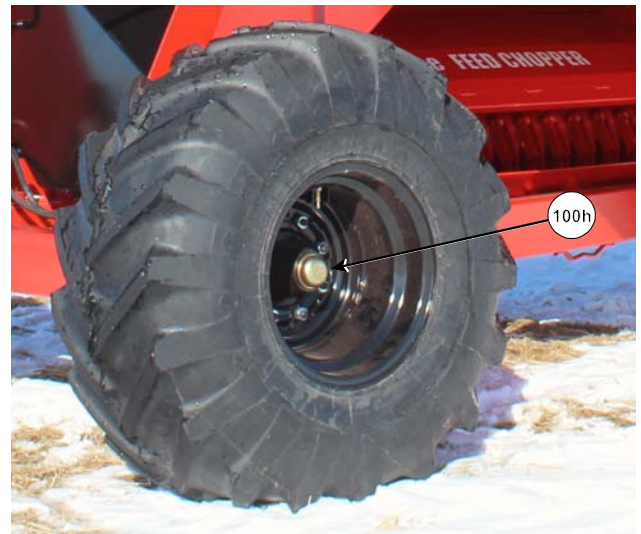
Grease Hubs on Both Spindles
