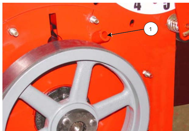
Remove the Flail Drum Lock Pin (Drive Shield Not Shown for Clarity)
