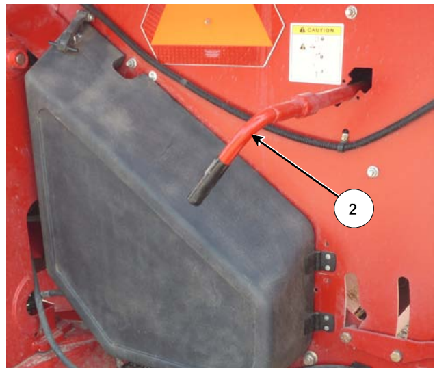
Remove Twine Cutter from Storage
