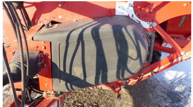
Ensure Driveline Shields are in Place
