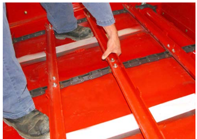
Check Tension of the Feeder Chain
