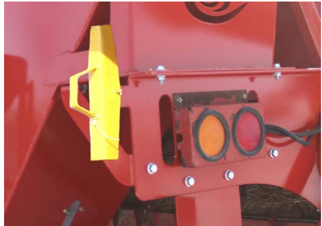
Cylinder Lock Stored (With Grain Tank)
