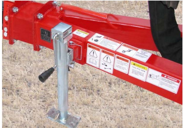
Jack on Hitch - Raise Hitch
