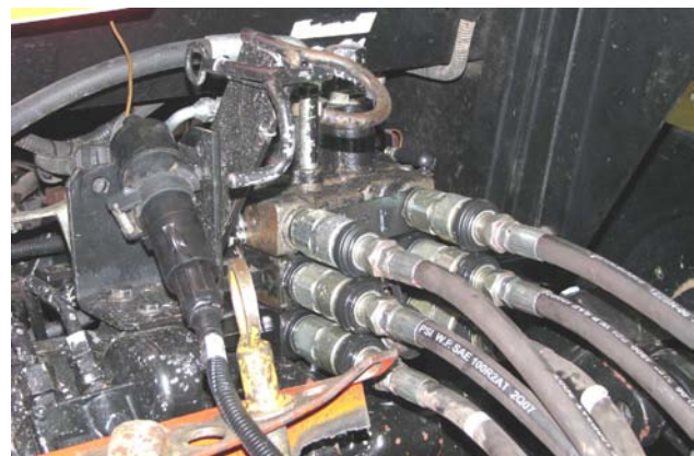
Disconnect Hydraulic Hoses & Electrical
