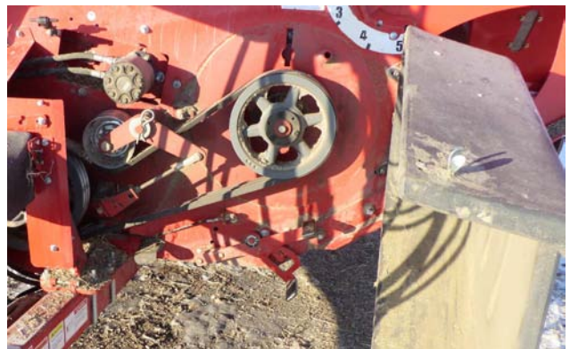
Open the Front Drive Shield - Check Belt
