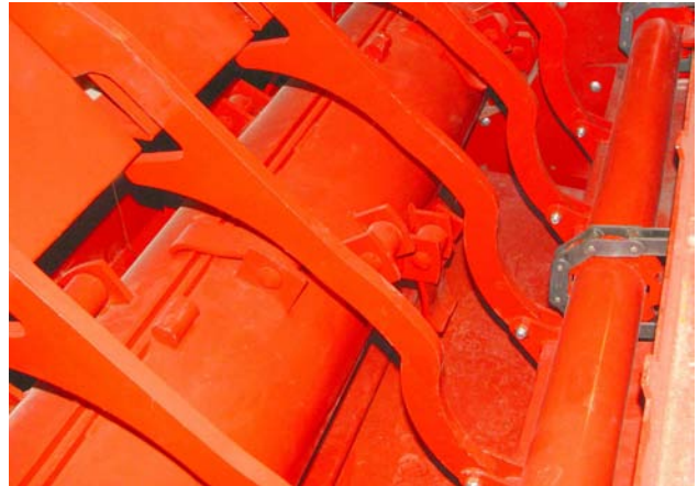
Move Flails Blocking the Knife Path
