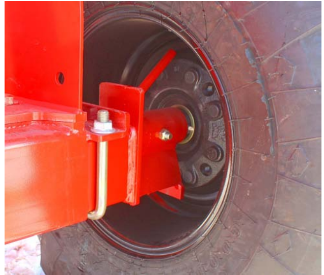
Remove Twine from the Spindle and Hub
