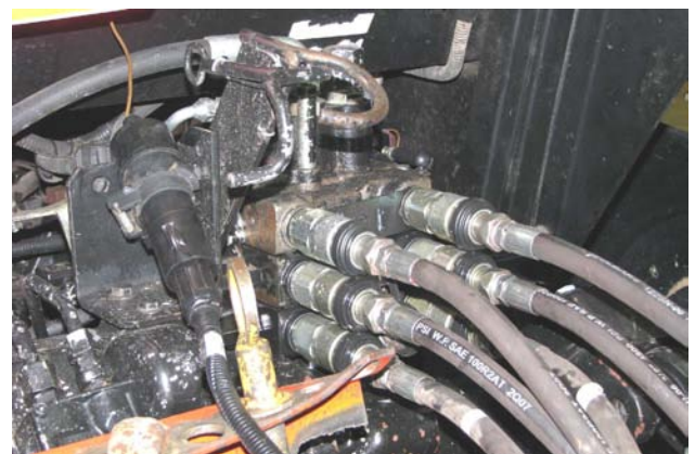
Inspect Hydraulic Hoses
