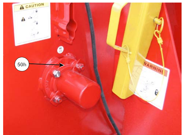
Grease Rear Flail Drum Bearing
