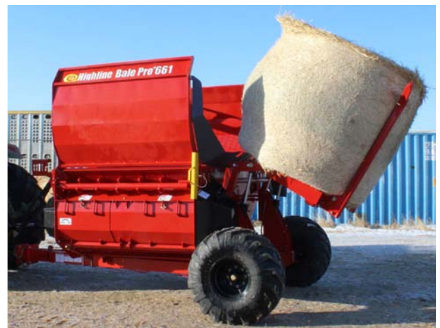
Raise Bale into Processor Tub
