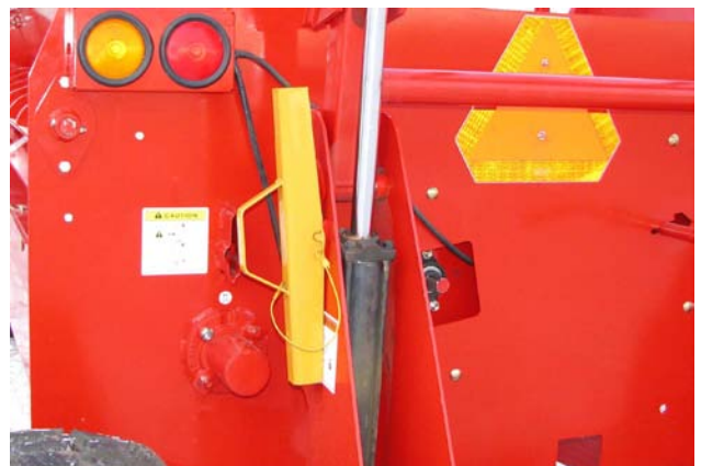
Remove & Store Cylinder Lock (No Feedchopper)
