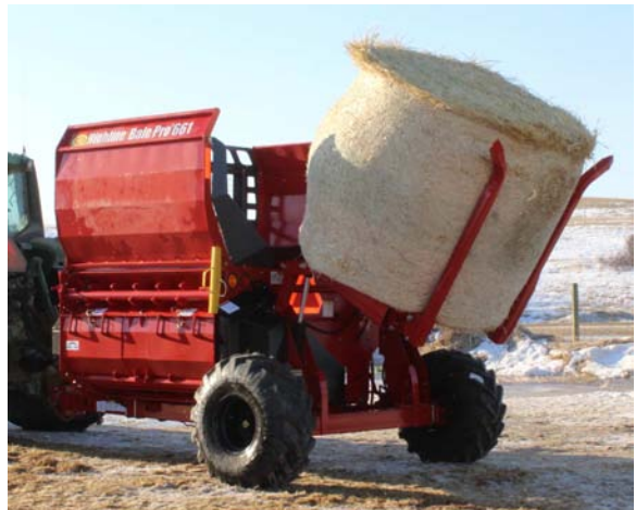
Stop the Feeder Chain When Loading
