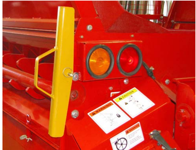
Cylinder Lock Stored (With Feed Chopper)
