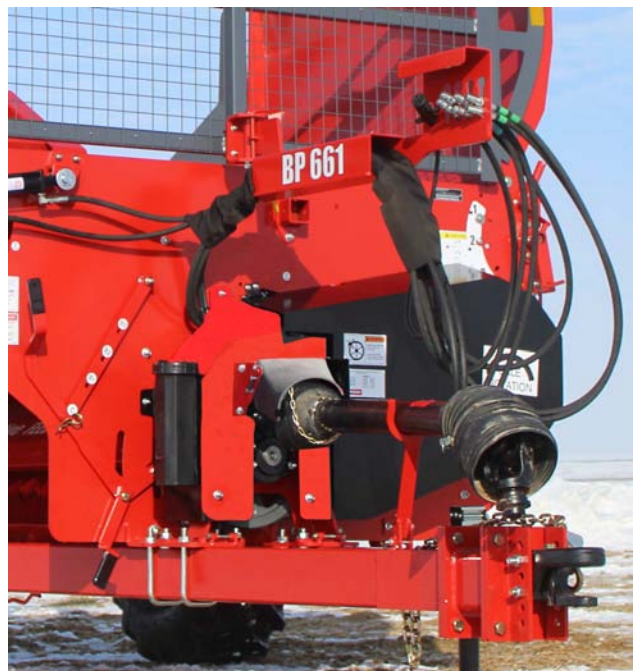
Remove Driveline and Safety Chain
