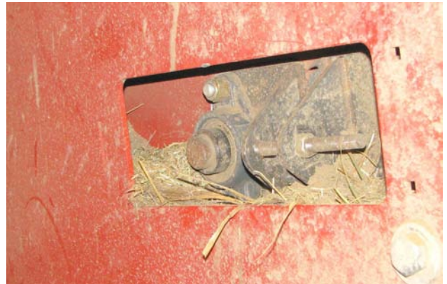
Remove Material - Upper Chain Bearing
