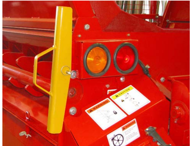
Cylinder Lock Stored (With Feed Chopper)
