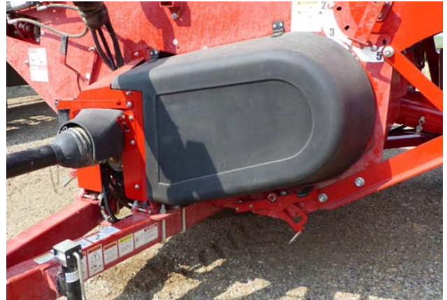
Ensure Driveline Shields are in Place
