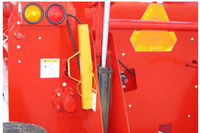
Remove & Store Cylinder Lock (No Feedchopper)
