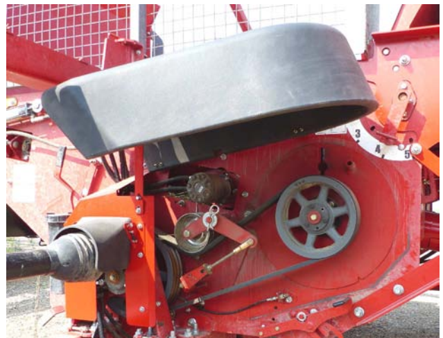
Open the Front Drive Shield - Check Belt
