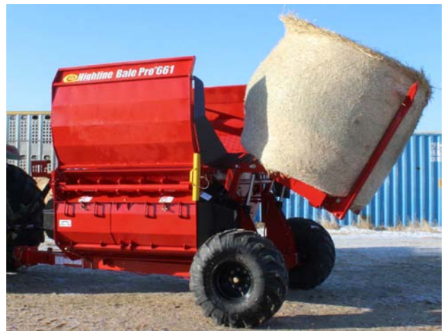
Raise Bale into Processor Tub
