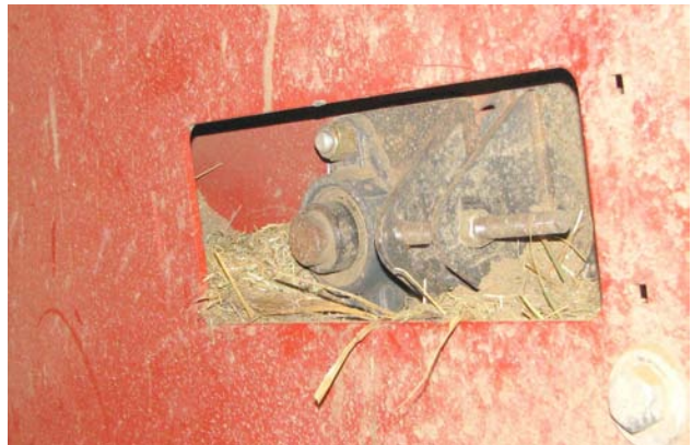
Remove Material - Upper Chain Bearing
