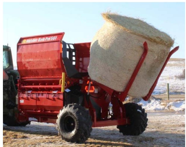
Stop the Feeder Chain When Loading
