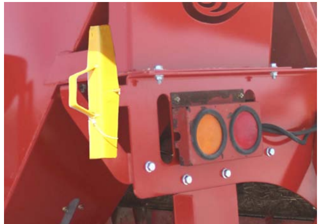
Cylinder Lock Stored (With Grain Tank)
