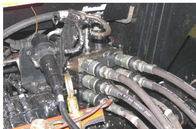
Disconnect Hydraulic Hoses & Electrical
