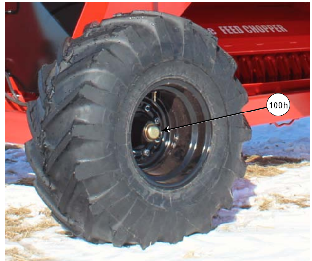
Grease Hubs on Both Spindles
