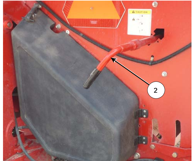
Replace Twine Cutter Into Storage Position
