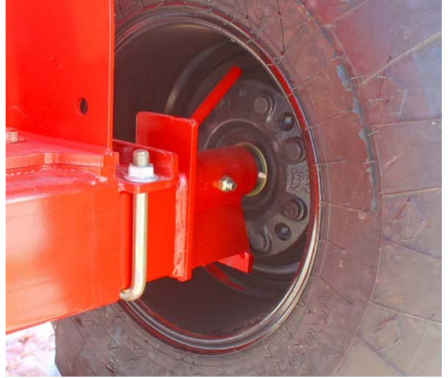
Remove Twine From the Spindle and Hub
