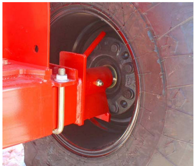
Remove Twine from the Spindle and Hub
