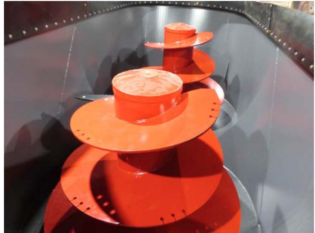
Check for Build Up in the Tub and the Condition of the Screws
