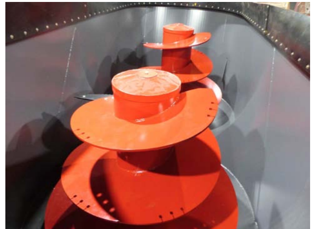
Remove all Material from the Tub
