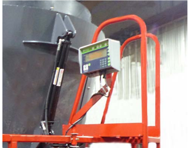
Monitor the Feeding Ration with the Weigh Scale Monitor
