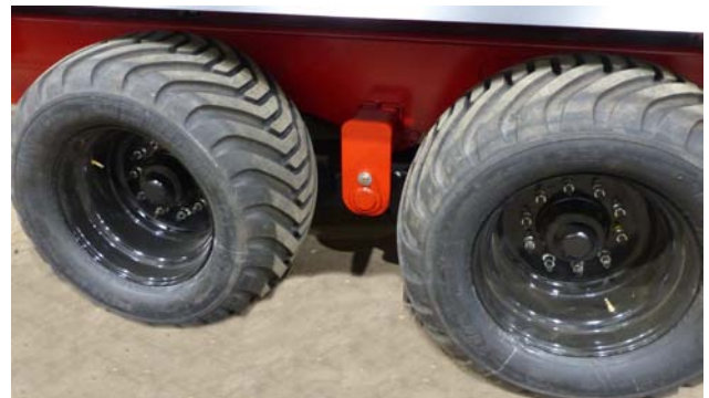
Place Jack Under the Spindle Tube of Tire to be Changed
