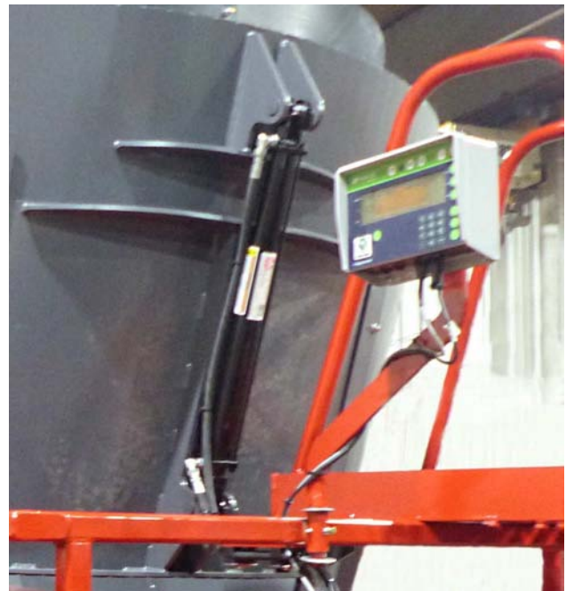
Inspect the Hydraulic Cylinder
