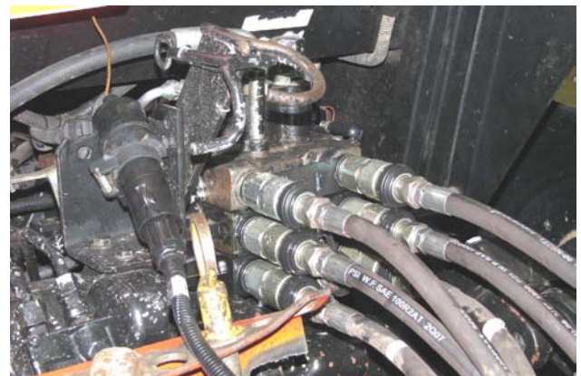
Disconnect Hydraulic Hoses & Electrical
