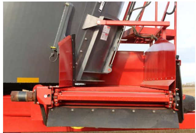
Check that the Unload Conveyor Works
