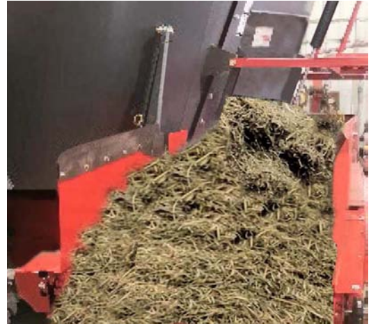
Open the Tub Door to Control Flow of Mixed Material
