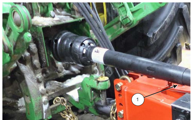
Connect the Driveline to PTO
