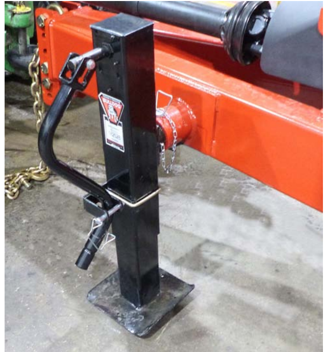
Lift Hitch with the Jack
