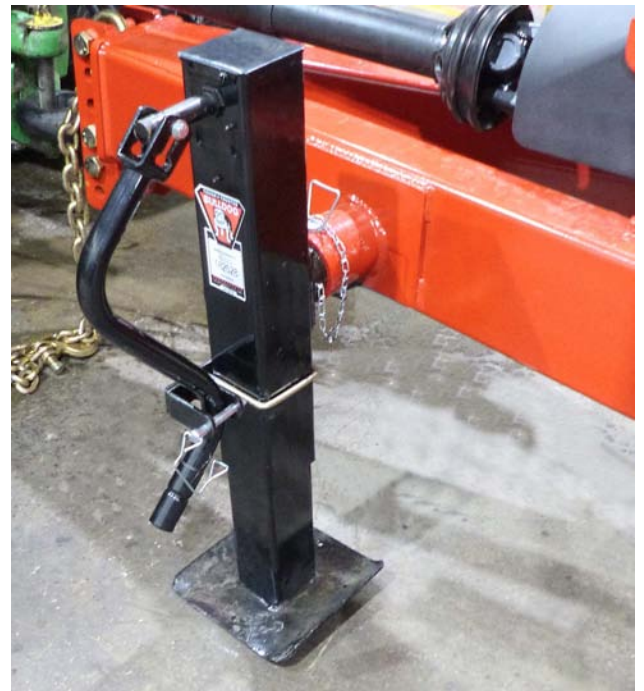
Lift Hitch with the Jack
