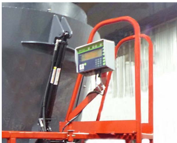
Monitor the Feeding Ration with the Weigh Scale Monitor
