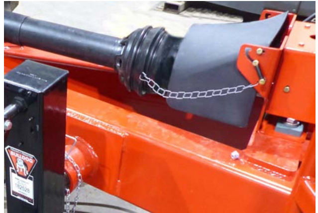
Connect Driveline Cover Chains
