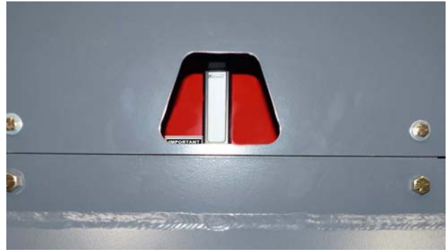
Check the Oil Level for the Mixing Screws
