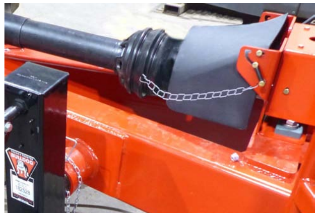
Connect Driveline Cover Chains
