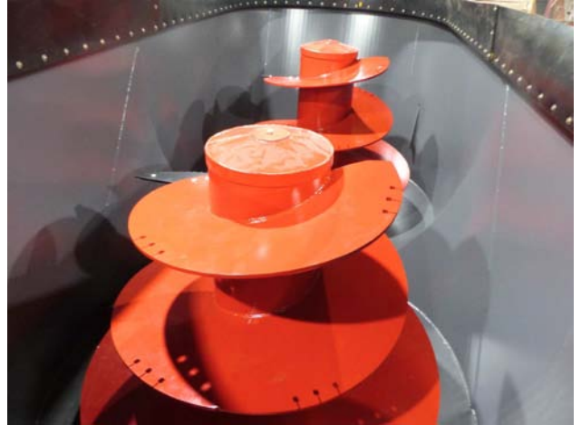
Turn Off Screws When Tub Is Empty
