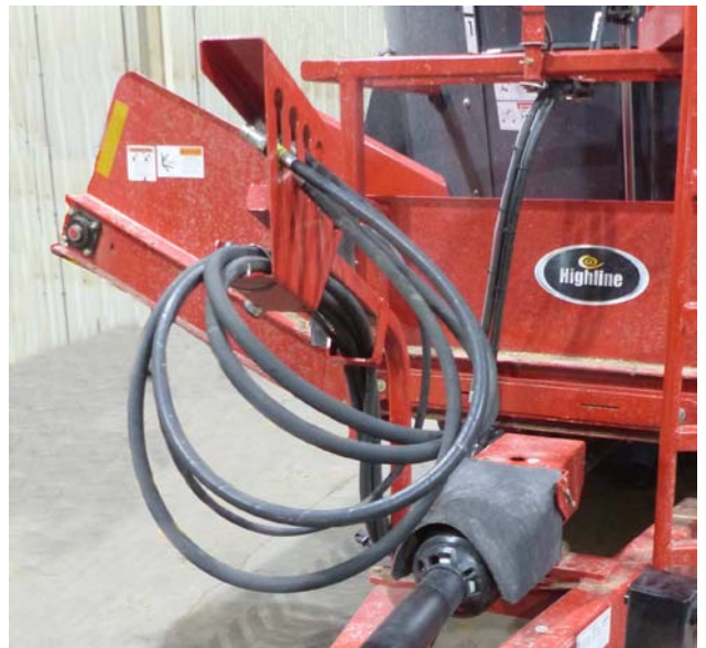
Place Hydraulic Hoses and Electrical Connector Into the Holder
