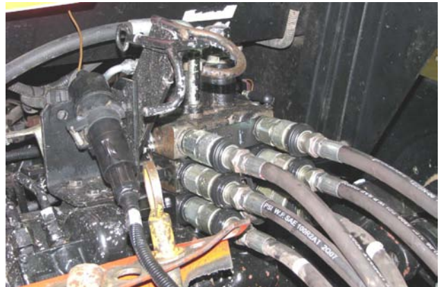
Disconnect Hydraulic Hoses & Electrical
