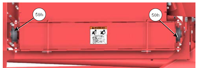
Grease Conveyor Rear Bearings
