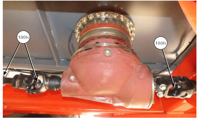
Front Screw Driveline (Comer Drivebox Shown)
