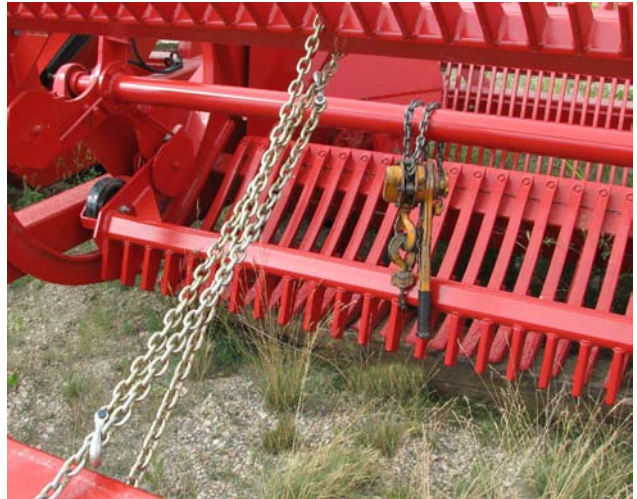
Winch The Lodged Bat-Remove Spring Pressure 108193
