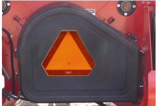
Install the Rear Upper Shield
