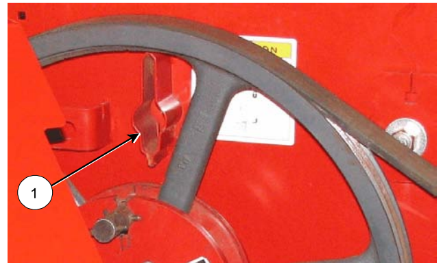
Align Sheave Spokes for Twine Cutter
