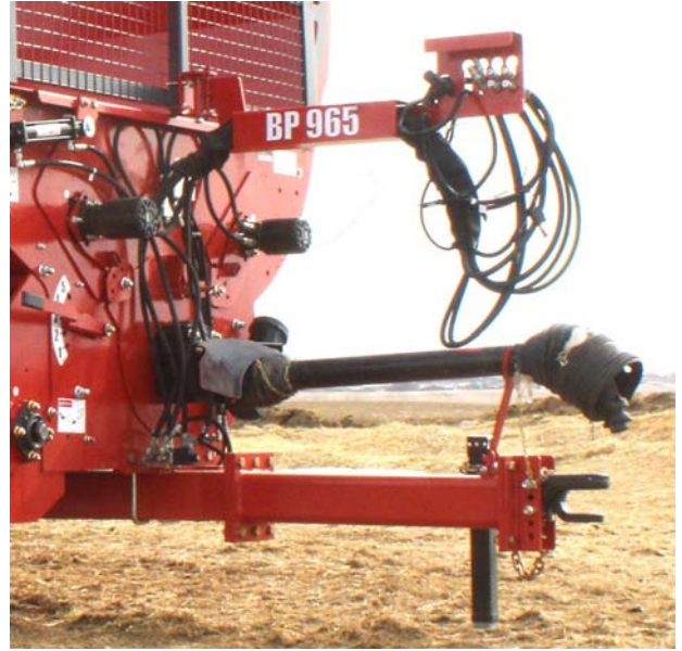
Route Hoses through Non-Abrasion Cover and through Hose Holder
