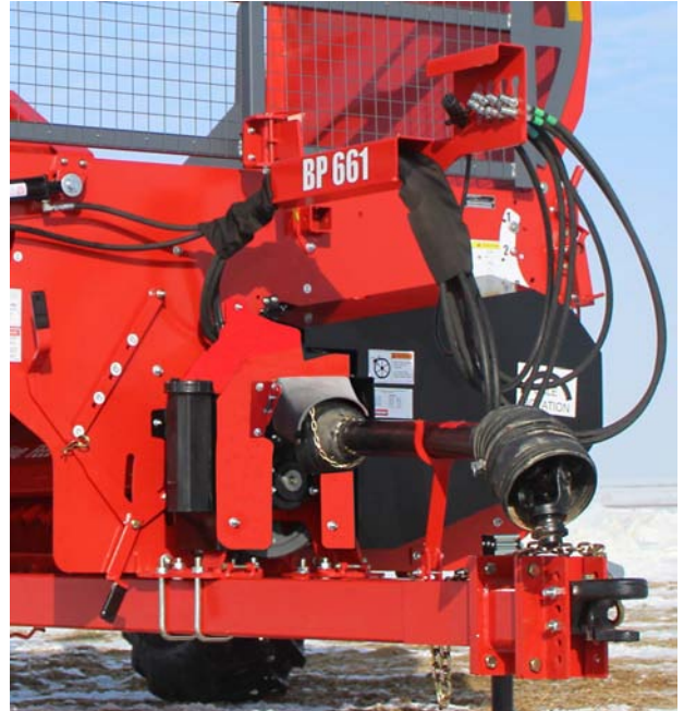
Route Hoses through Non-Abrasion Cover and through Hose Holder
